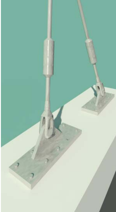
Fig. 9: Details of the hanger and slab connection
