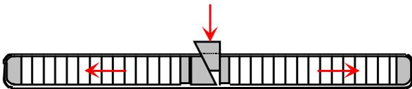
*Fig. 4: Principle of the application of the lateral prestressing of the glulam slab with the help of wedges. The prestressing had to be conducted iteratively over the length of the slab and the wedges were glued-in at the final stage. The grey shaded parts ideally are made of hardwood in order to minimize the effect of possible indentations in the wood. In our case only the two outer lamellas were made of oak.*
