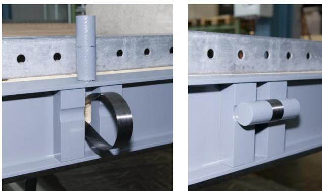
Fig. 8: Anchoring of the longitudinal tension loops at the plate's front end using a GFRP bolt with a diameter of 4 cm. This diameter is towards the lower end of possible bending radii for the used CFRP elements that can be realized in practice without damaging the CFRP structure. The fixation of the bolt as well as the profile that covers the front end of the plate and serves to distribute the loads originating from the loops into the slab are made of GFRP.
