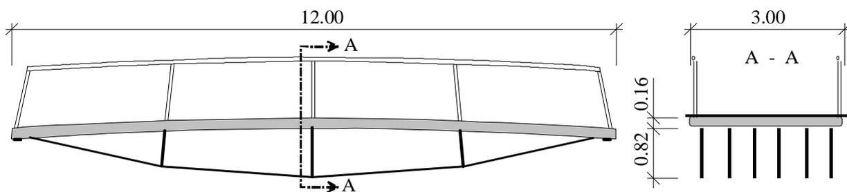
Fig. 2 Overview of the bridges design and main dimensions
