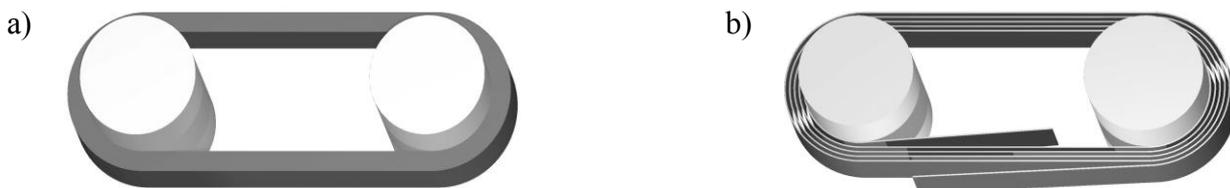
Fig. 3: Principal design of pin loaded strap elements (loops), a) laminated CFRP, b) not laminated CFRP tapes.
