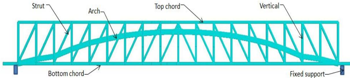
Fig. 8 STAAD model of the Cox Ford Bridge
