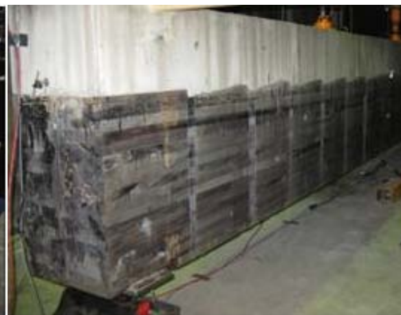
Fig. 6. Test arrangement and the wood-concrete composite test beam.
