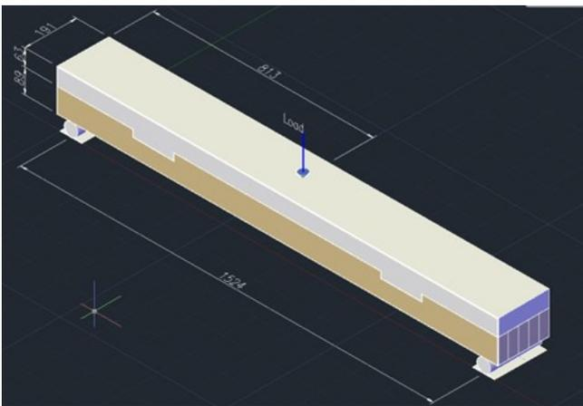
Fig. 1 Specimen configuration [mm]
