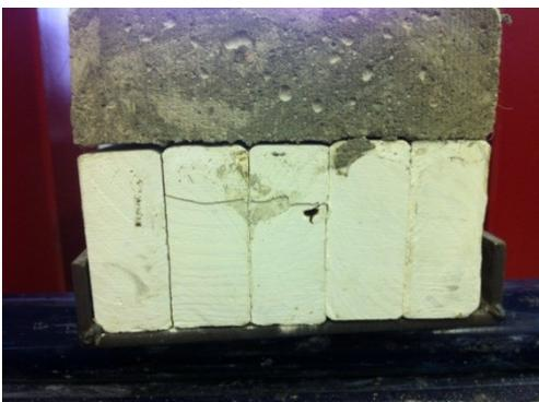
Fig. 5 Typical block-shear failure
