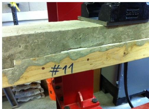
Fig. 6 Typical tension failure
