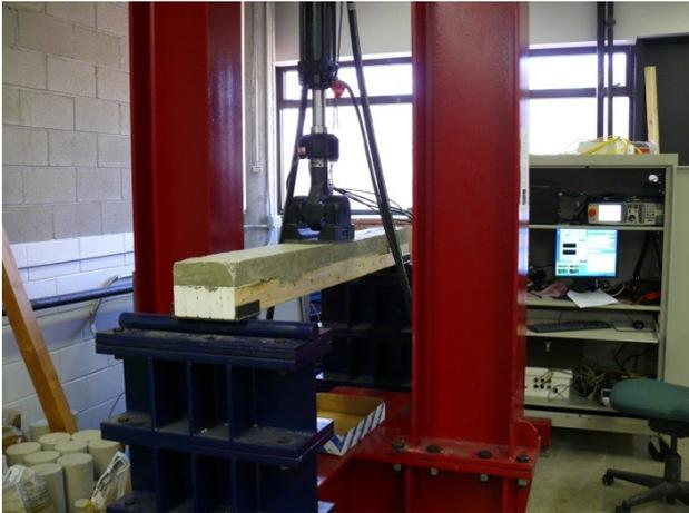
Simply supported specimens were configured with a span of 1524 mm (60 in). Mid-span (three-point loading) loading was applied using an MTS hydraulic loading and digital data acquisition system. Roller supports were configured at each end to avoid horizontal forces straining the actuator, resulting in a symmetric configuration, see Fig. 2. Some of the specimens were subject to static loading while others to cyclic pulsating loading.
