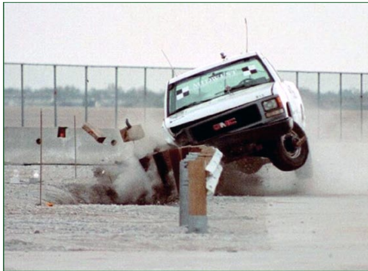
Full-scale crash test of wood post guardrail system.
