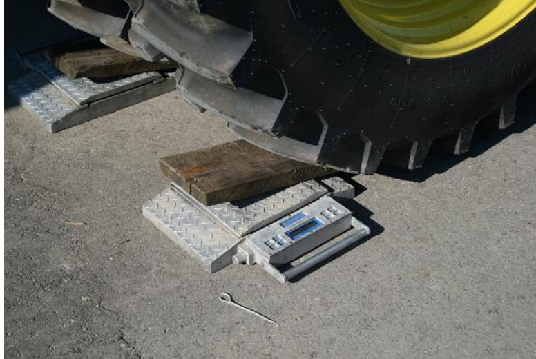
Figure 3.16. Weighing vehicles using portable scales
