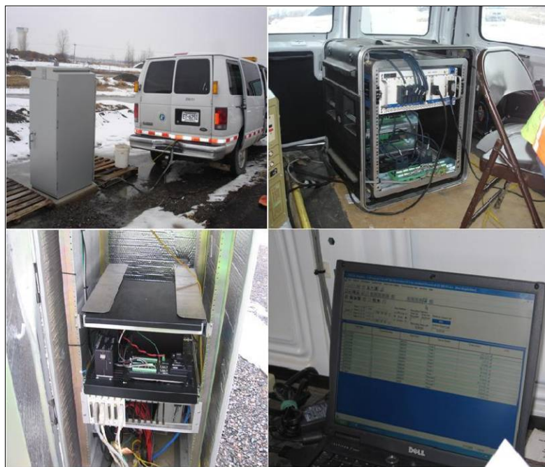
Figure 3.14. MnROAD pavement response data collection system
