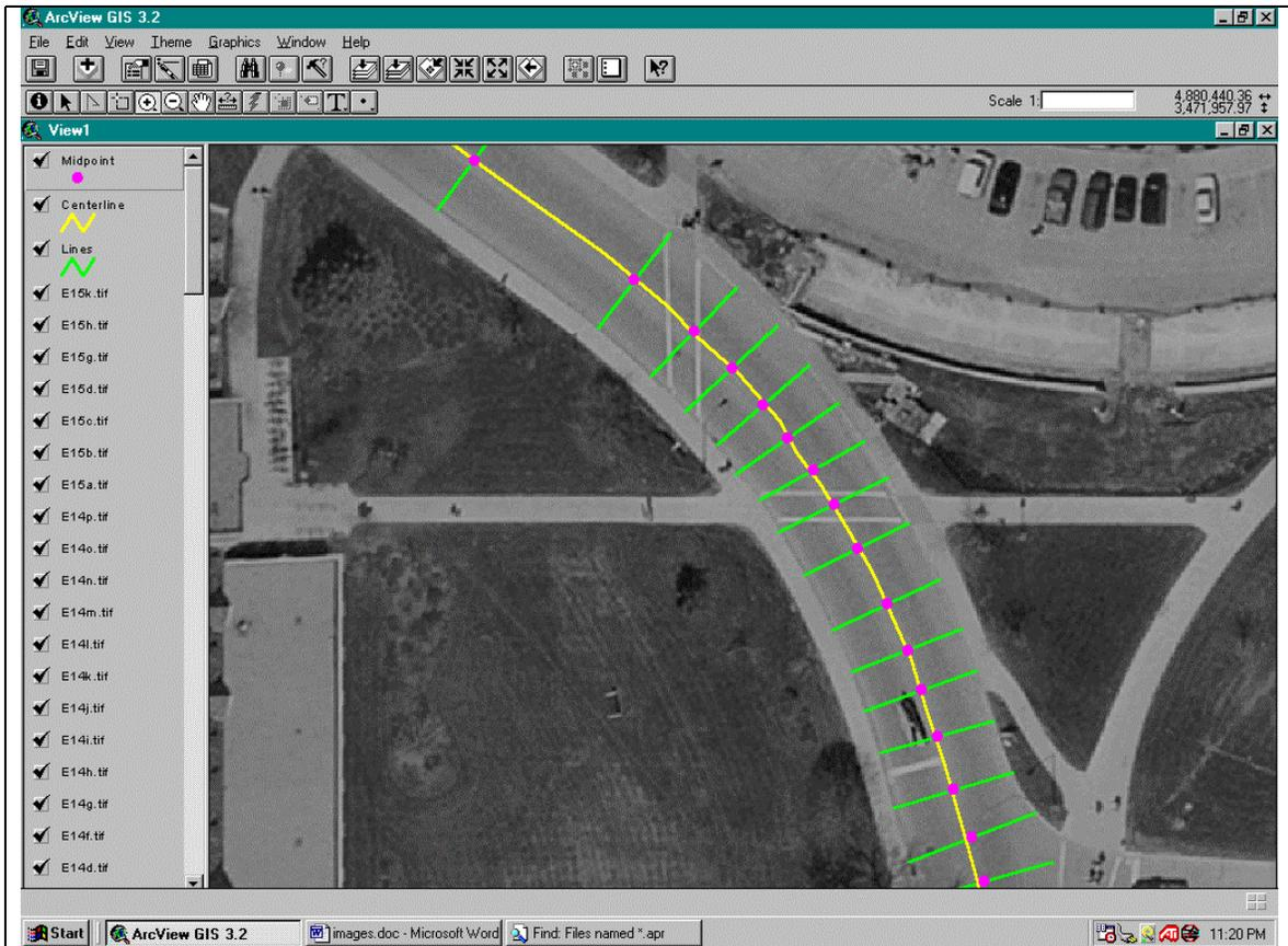
**Figure 7. Calculation of Roadway Centerline**
