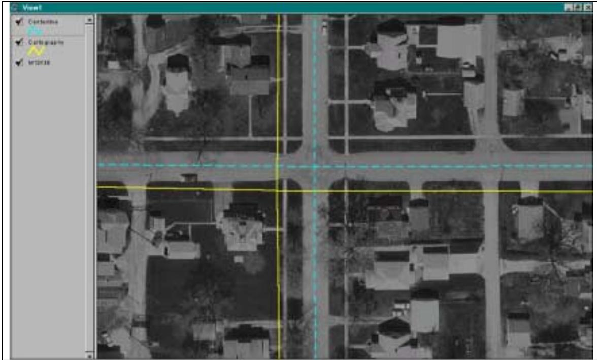
**Figure 13. Cartography Alignment Error**
