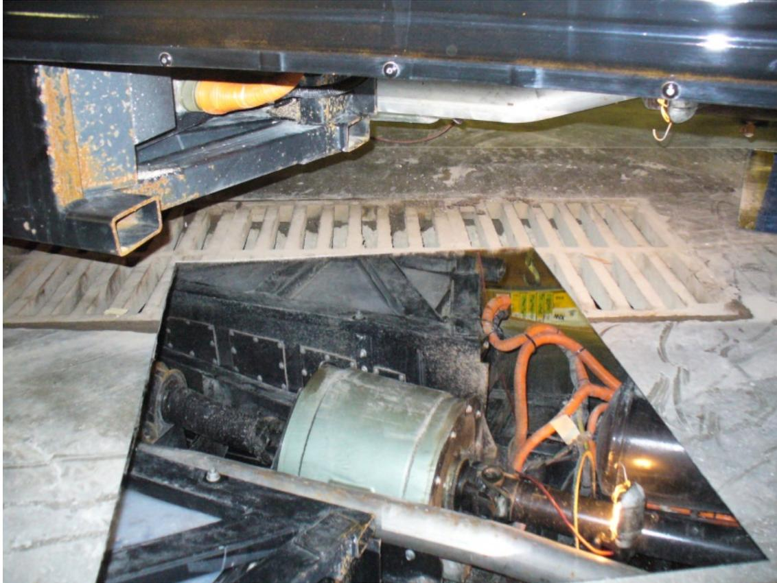
**Figure 3-5: Power train for one of Iowa’s hybrid-electric school buses**
