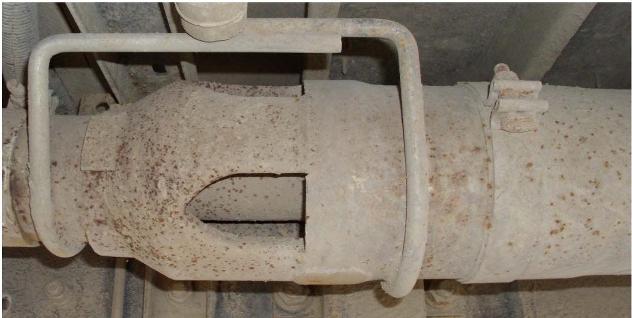
**Figure 5-1: Tailpipe Configuration on Hybrid School Bus**
