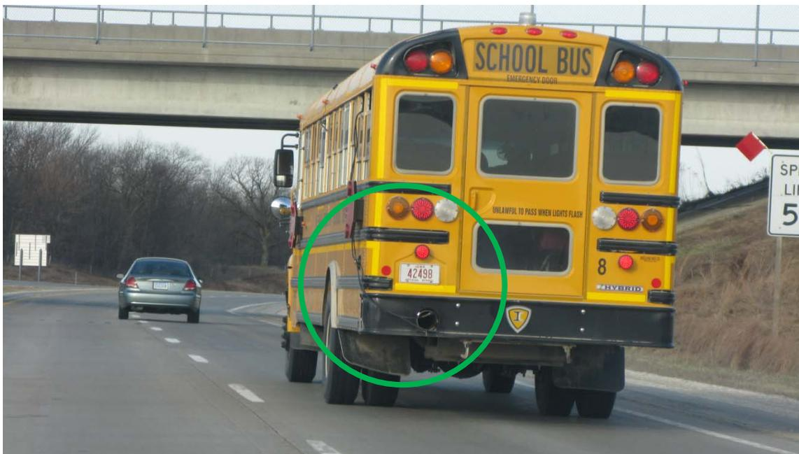
**Figure 5-4: Conducting On-road Testing (tailpipe probe circled)**
