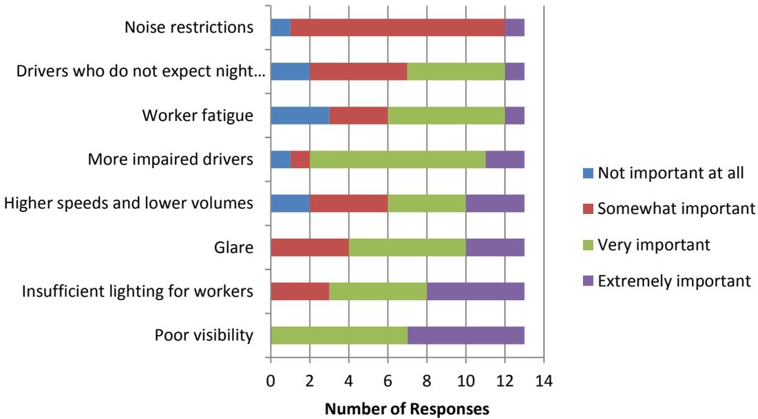
**Figure 3.20. Significance of the different risks in nighttime work-zone traffic control**
