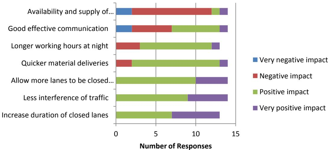
**Figure 3.18. Factors affecting nighttime construction productivity**
