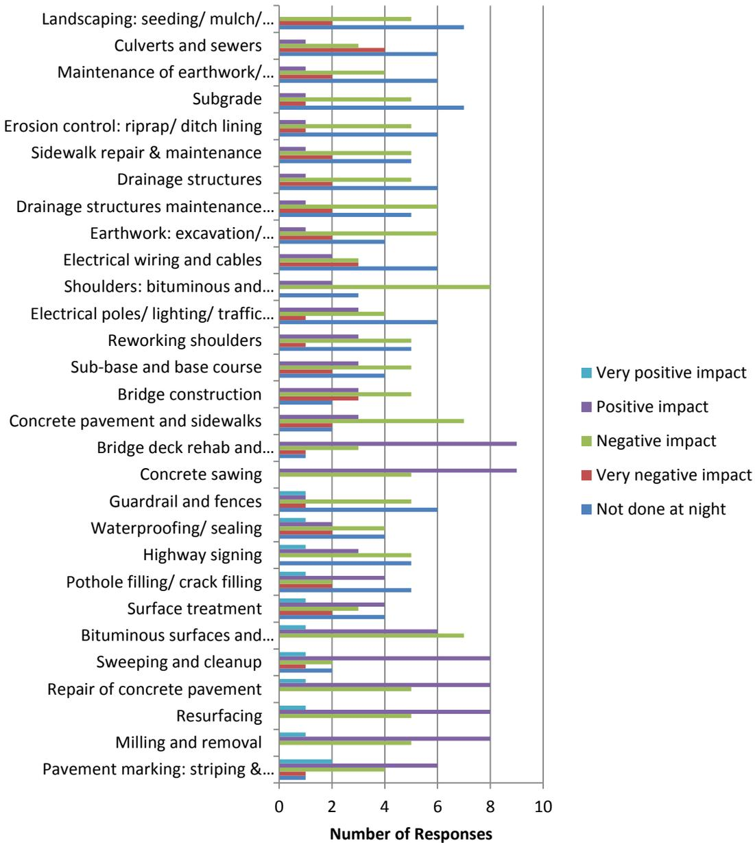
**Figure 3.19. Nighttime construction impacts on activity productivity**
