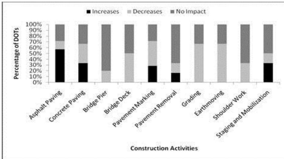
**Figure 4.9. Impact of nighttime construction on activity productivity**
