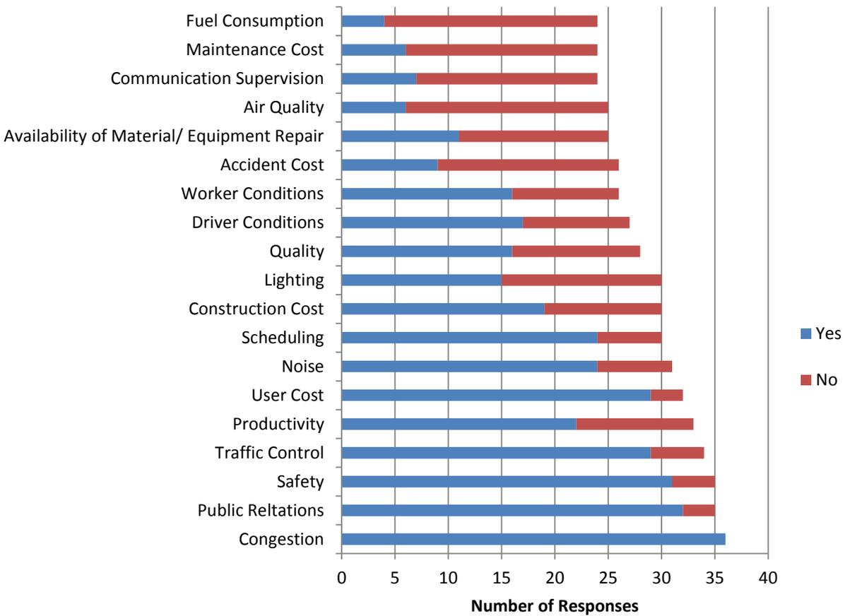
**Figure 3.4. Factors that affect choice of using nighttime construction**
