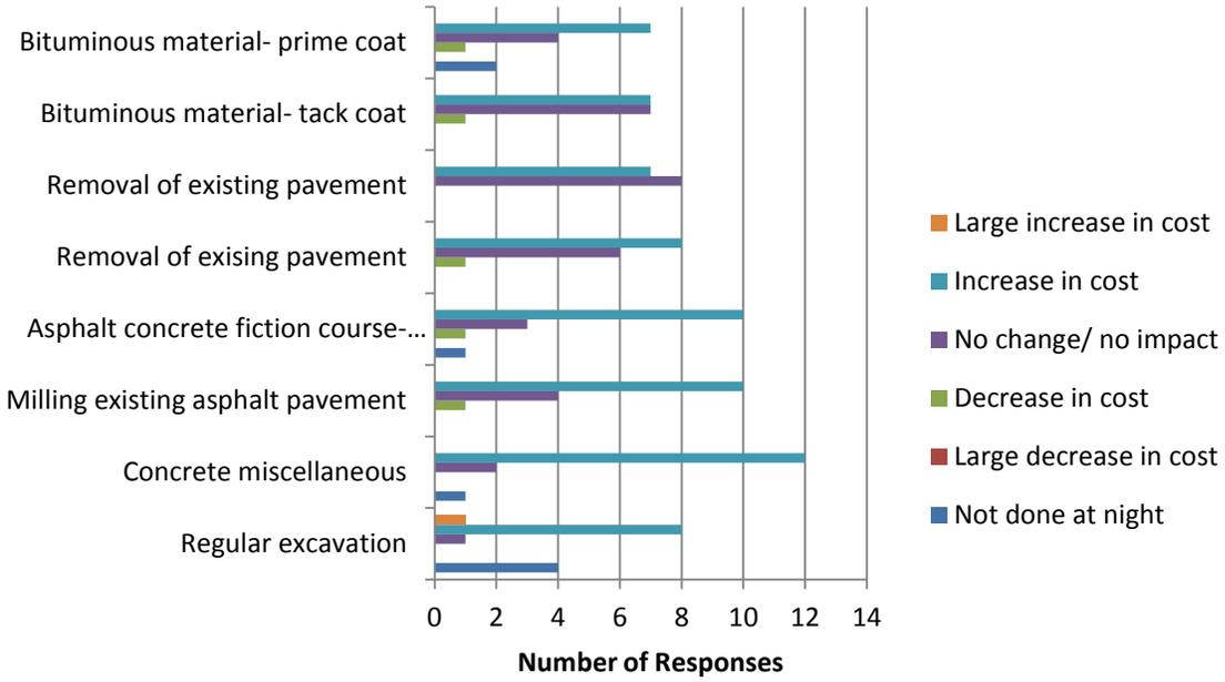
**Figure 3.24. Increases in construction cost for nighttime activities**
