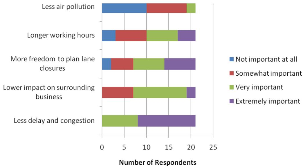
**Figure 3.6. Respondent opinions on the advantages of performing nighttime work**
