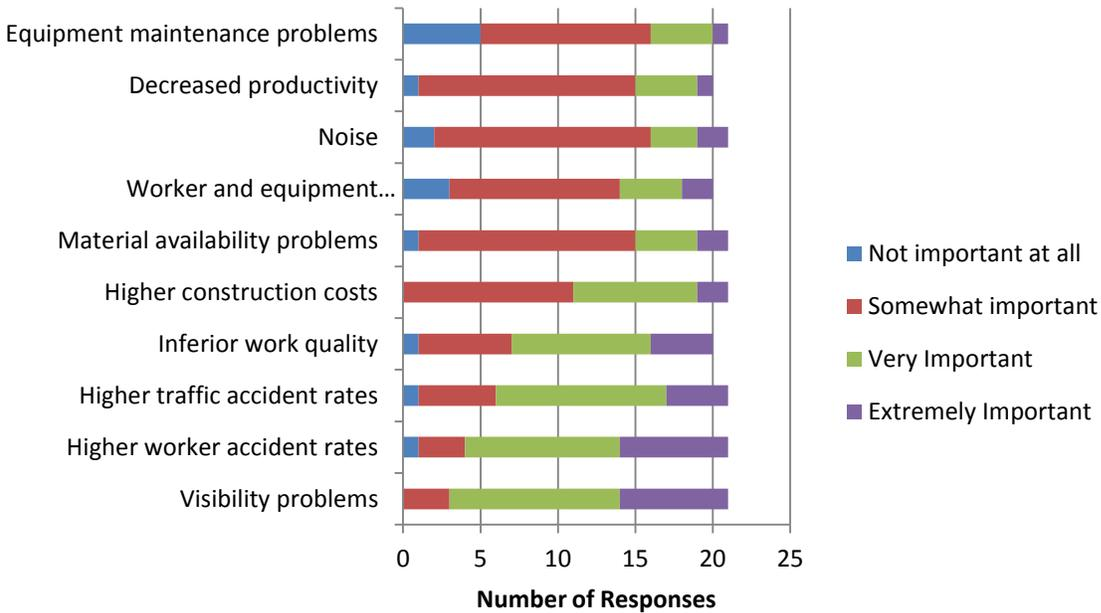
**Figure 3.7. Respondent opinions on the disadvantages of performing nighttime work**
