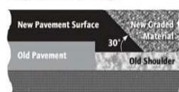
The Safety Edge is created by a custom pan installed on the paver to create a 30-degree consolidated wedge.
