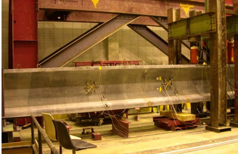
Figure 4.13. Large-scale flexure-shear test setup photograph.
