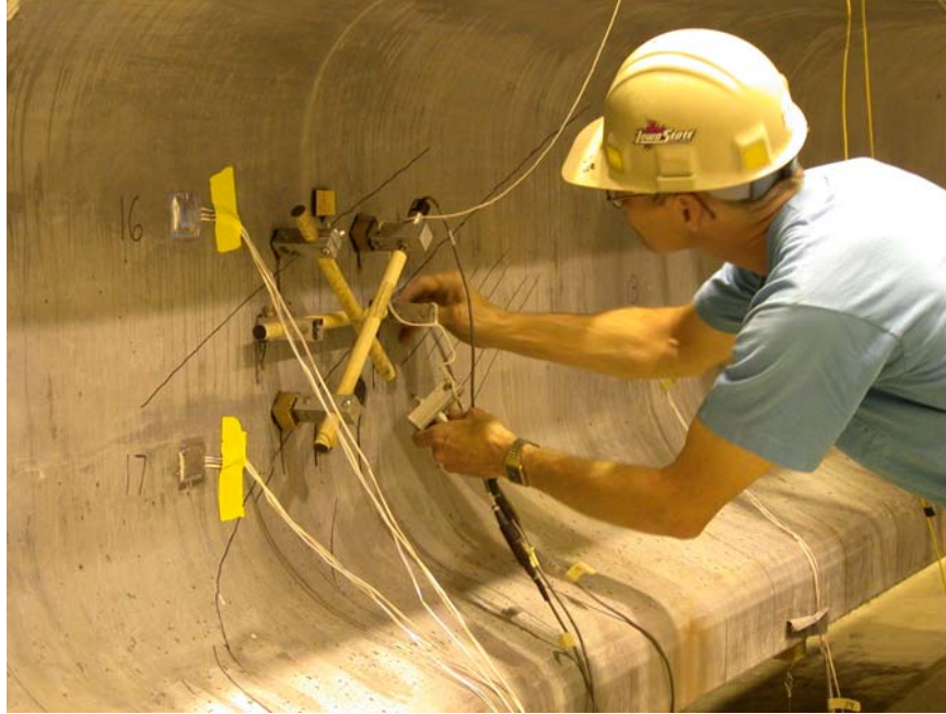
Figure 6.16. Flexure and shear cracking near gage R1 at a total load of 482 kips during the large-scale flexure-shear test.
