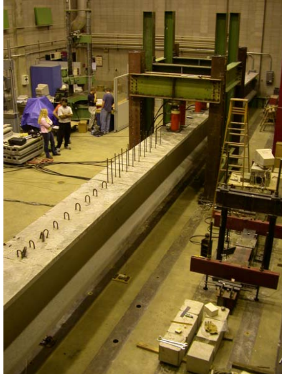
Figure 4.4. Large-scale flexure test setup photograph.
