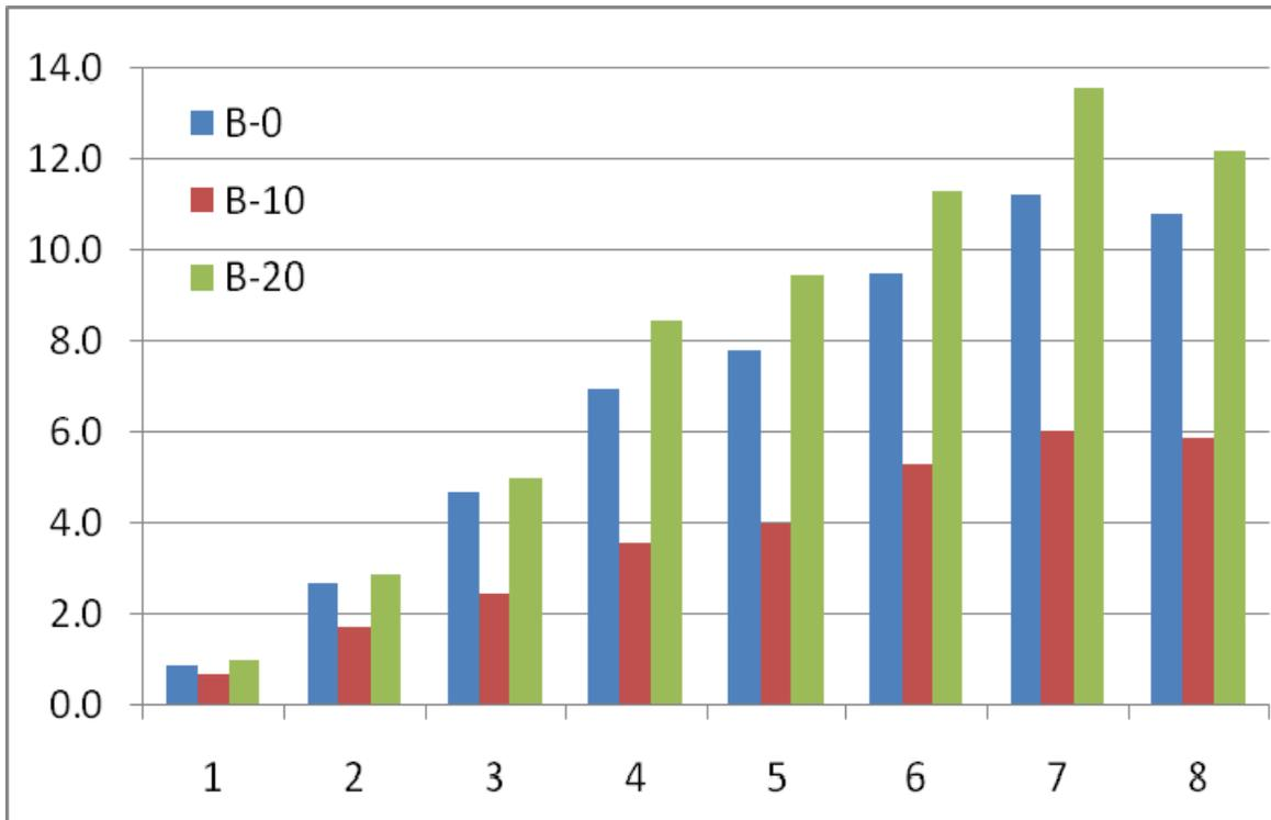
Figure 3-25. CO<sub>2</sub> emissions for Bus 971 by VSP bin
