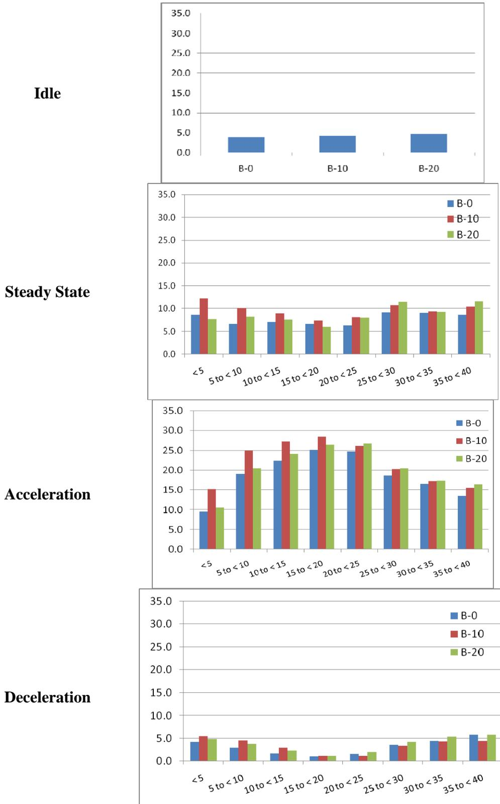
Figure 3-36. CO<sub>2</sub> emissions (g/s) for Bus 997 by mode and speed (mph)
