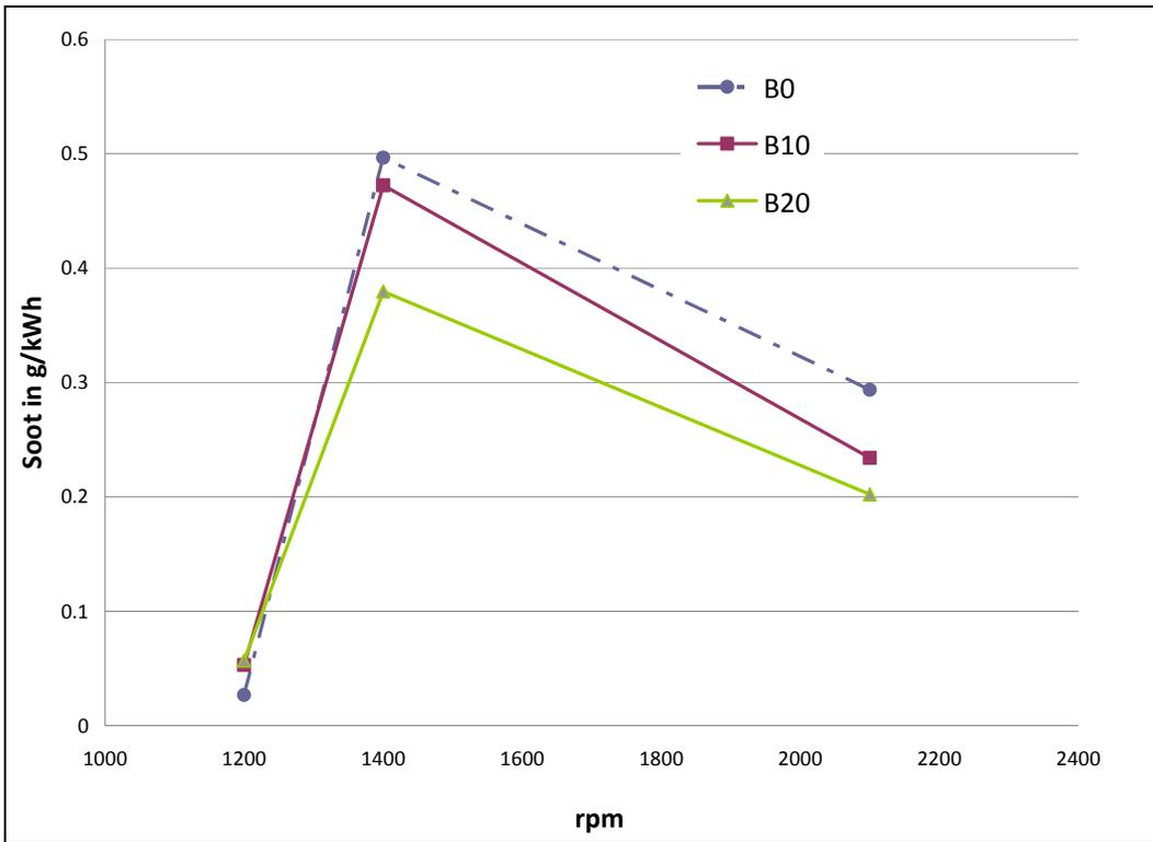
**Figure 4-4. Soot emissions corresponding to each operating conditions**
