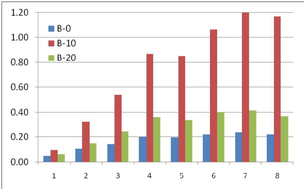
**Figure 3-38. PM emissions (mg/s) for Bus 997 by VSP bin**
