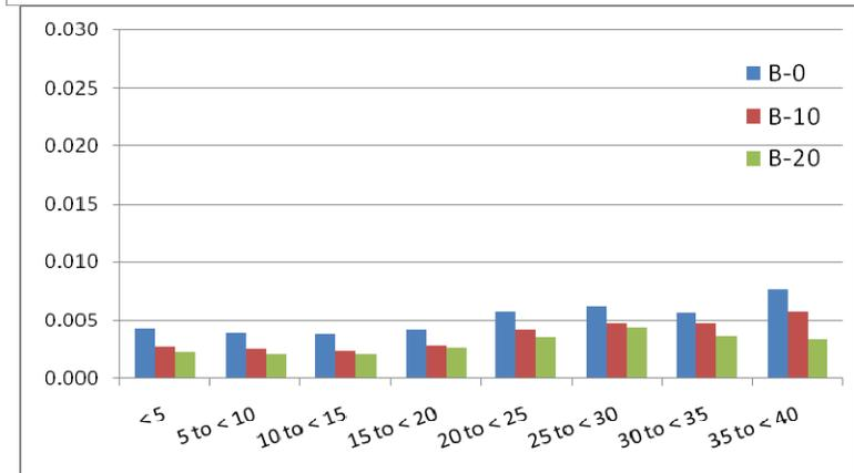
**Figure 3-33. CO emissions for Bus 997 by mode and speed (mph)**
