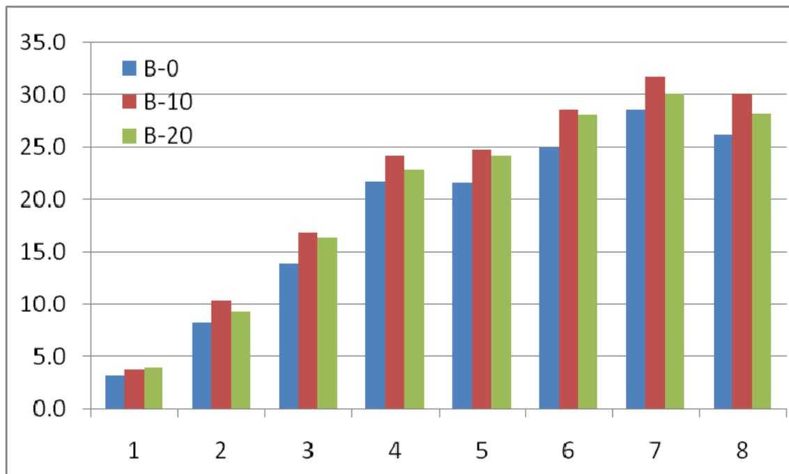
**Figure 3-35. CO<sub>2</sub> emissions (g/s) for Bus 997 by VSP bin**
