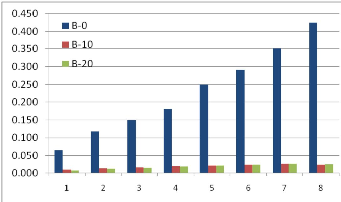
**Figure 3-28. PM emissions (mg/s) for Bus 971 by VSP bin**
