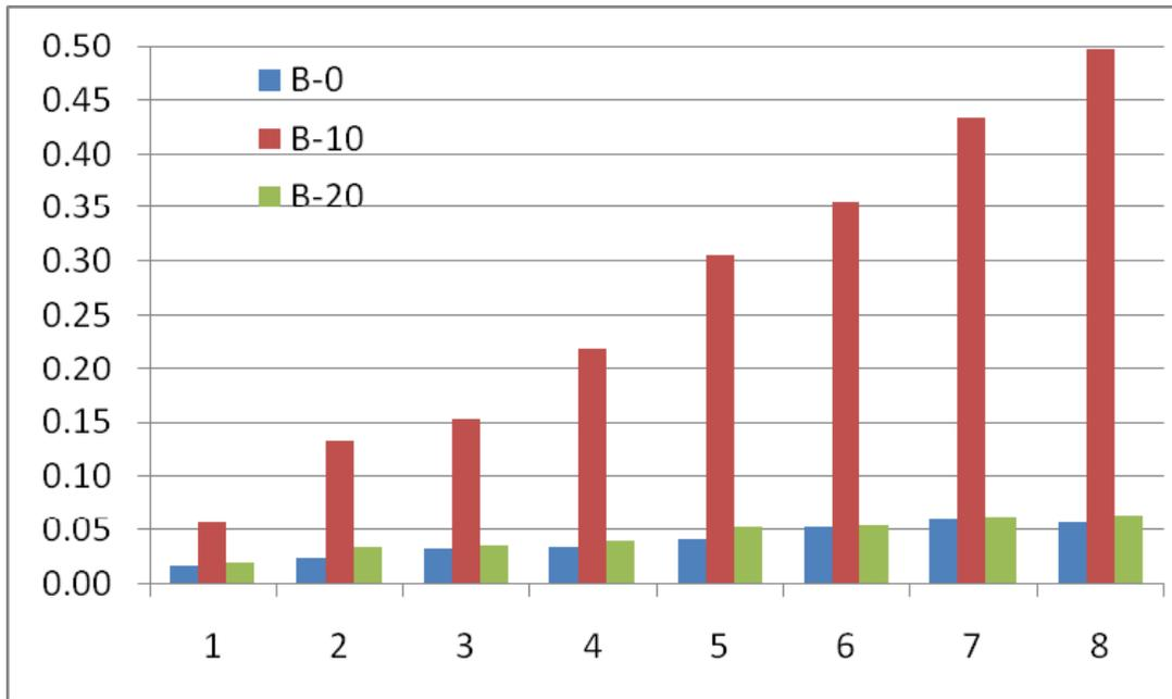
**Figure 3-18. PM emissions (mg/s) for Bus 973 by VSP bin**
