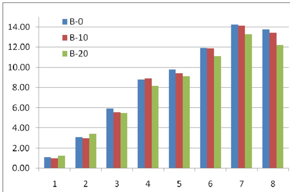
**Figure 3-15 CO<sub>2</sub> emissions (g/s) for Bus 973 by VSP bin**
