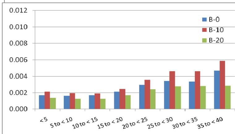
**Figure 3-32. HC emissions for Bus 997 by mode and speed (mph)**
