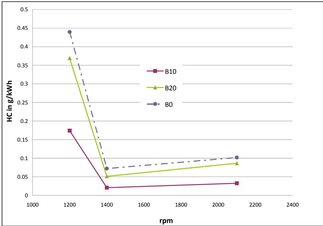
**Figure 4-6. HC emissions corresponding to each operating conditions**
