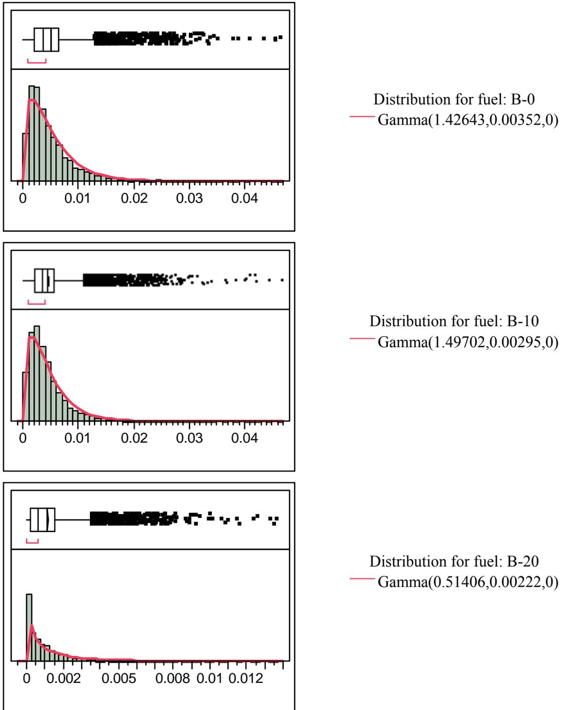
**Figure 3-8: Fitted gamma distributions for Bus 973 in acceleration by fuel type**
