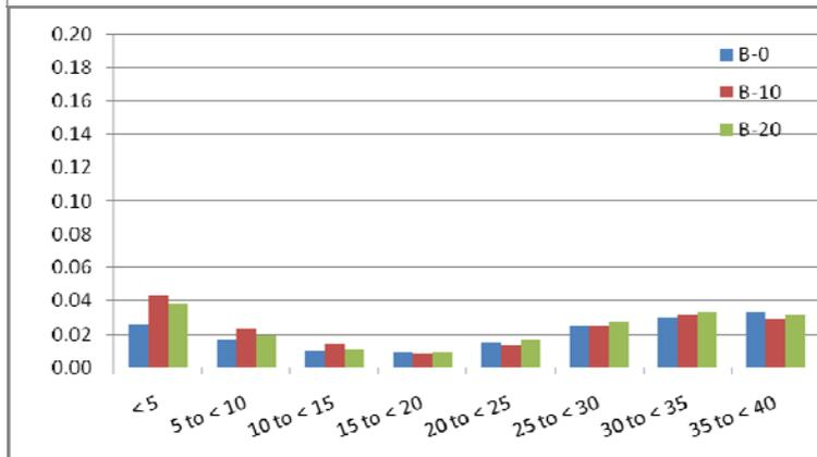
**Figure 3-29. NO<sub>x</sub> emissions (g/s) for Bus 997 by mode and speed (mph)**
