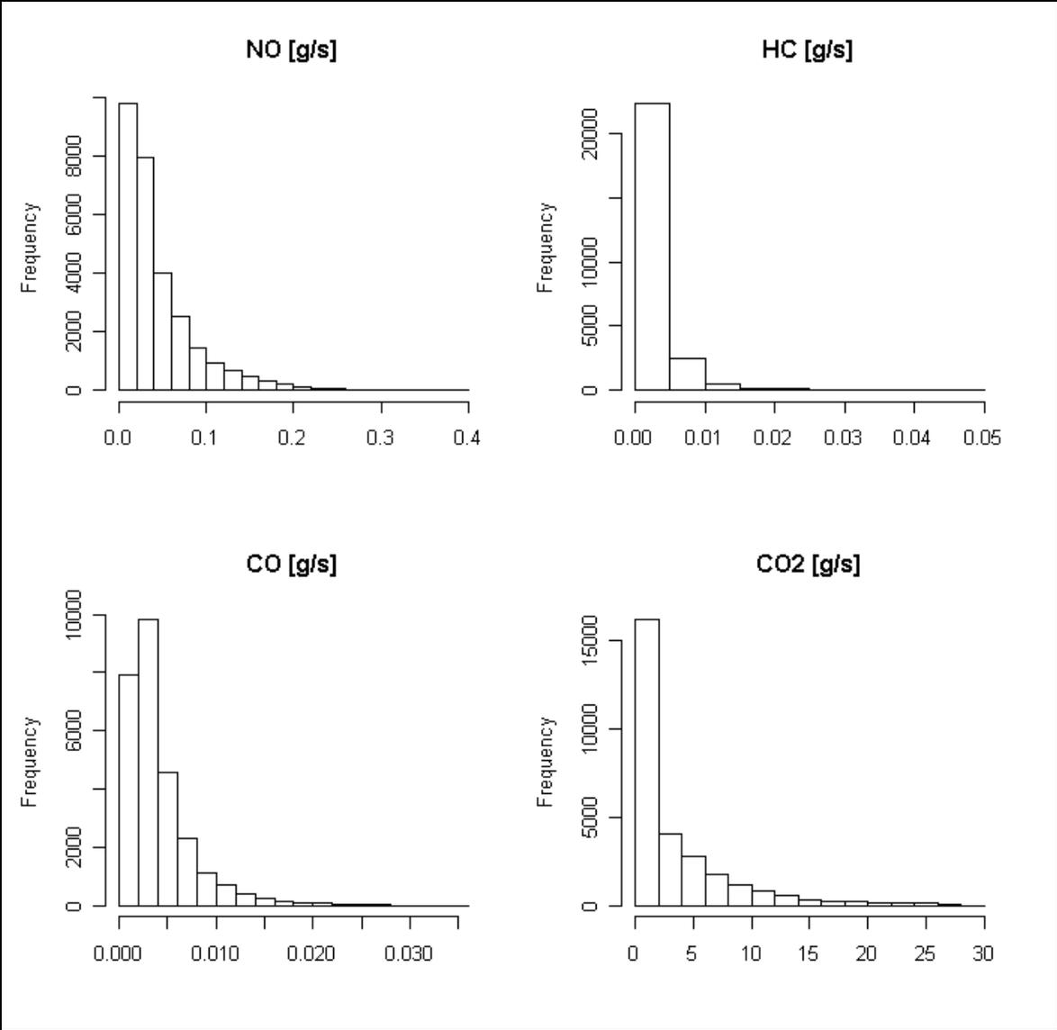
**Figure 3-7. Histograms showing conditional distribution by pollutant for Bus 973**
