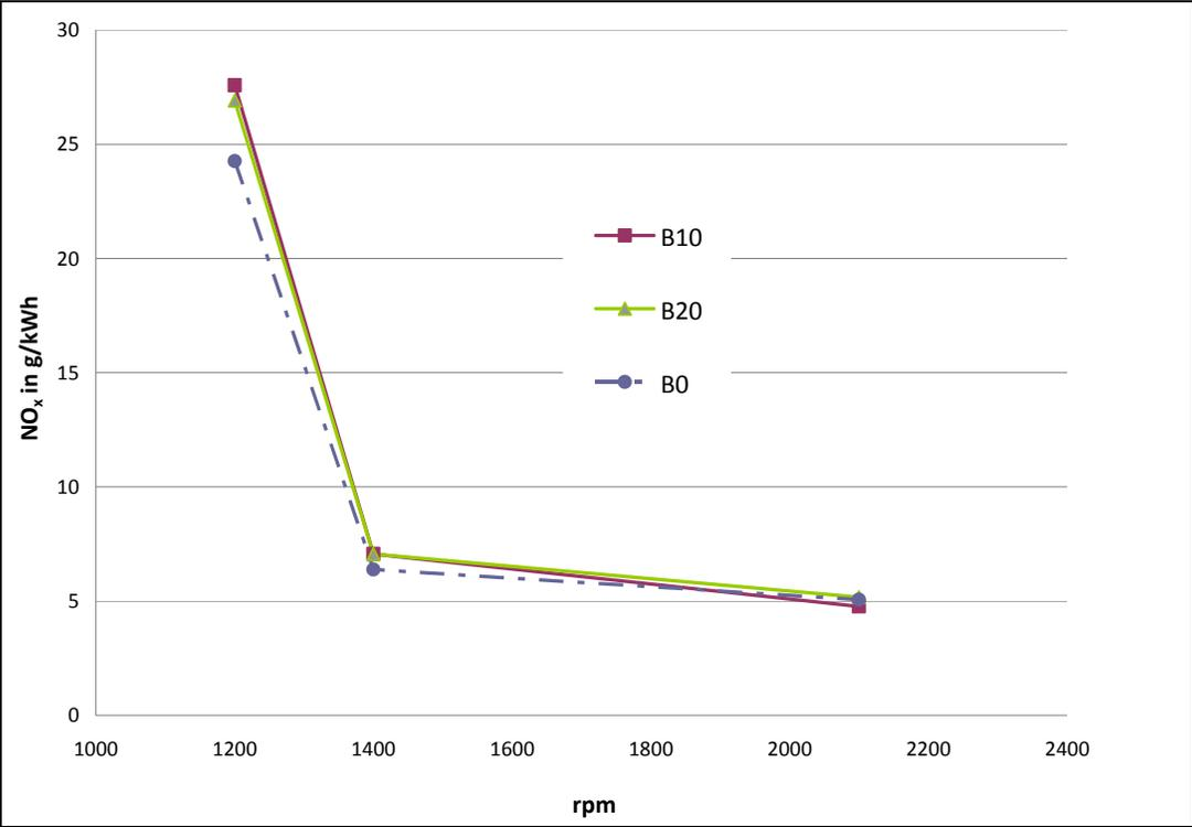
**Figure 4-3. NOx emissions corresponding to each operating condition**
