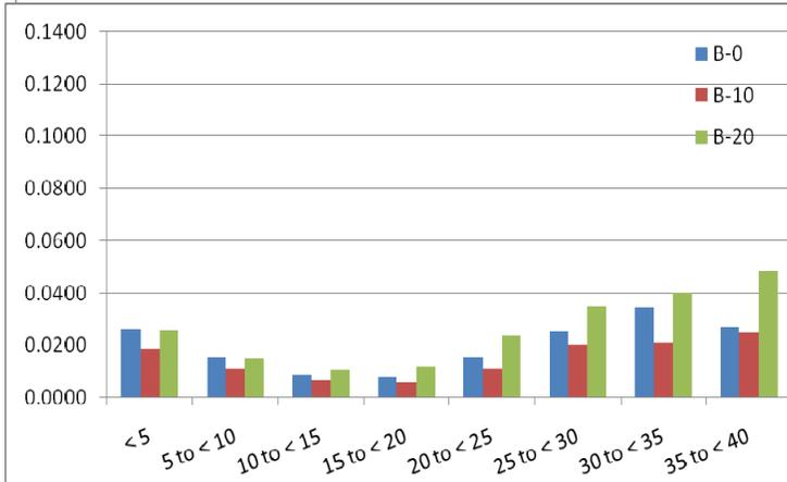
**Figure 3-9. NO<sub>x</sub> Emissions (g/s) for Bus 973 by Mode and Speed (mph)**
