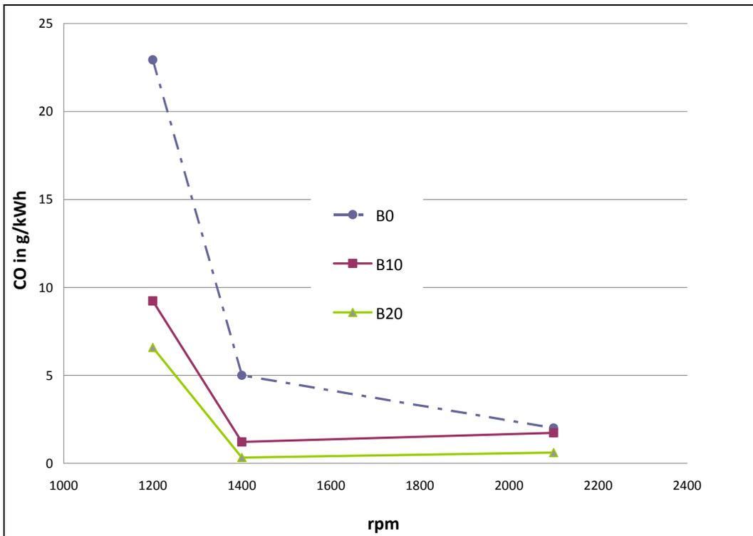
**Figure 4-5. CO emissions corresponding to each operating conditions**
