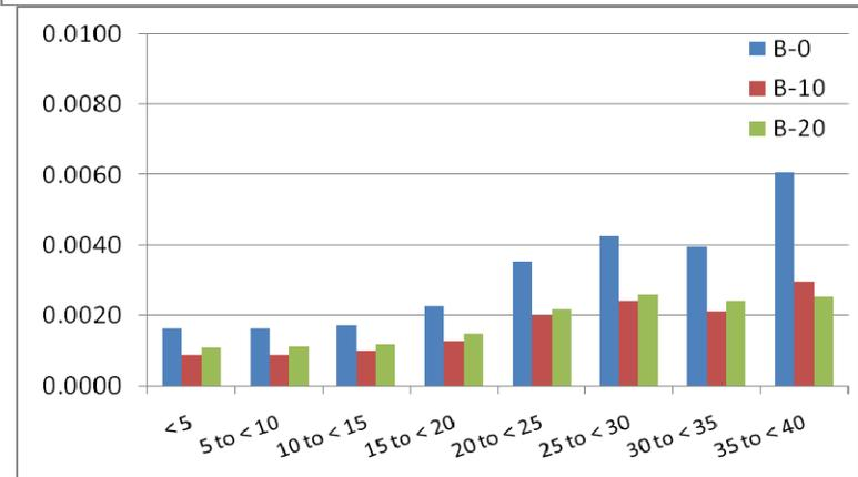
**Figure 3-13: CO Emissions (g/s) for Bus 973 by Mode and Speed (mph)**
