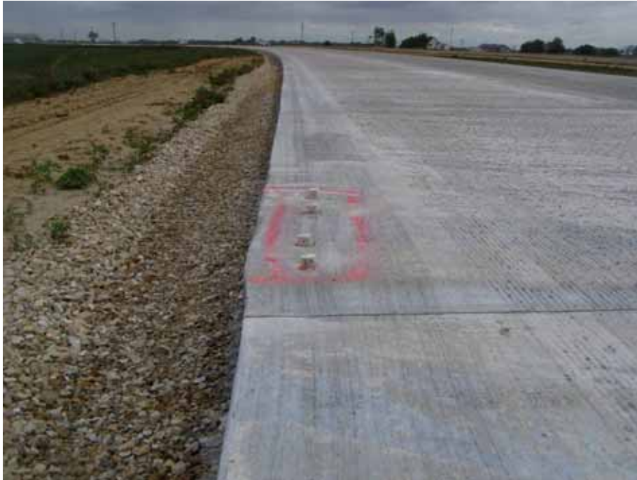
Figure D.11. Relative humidity instrumentation location
