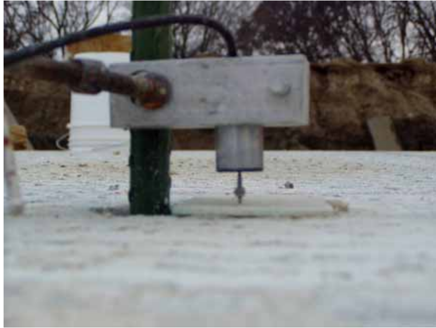
Figure 23. Typical LVDT installation (Iowa State)
