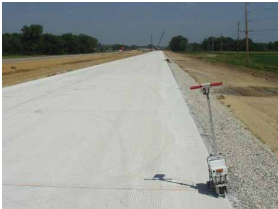
Figure G.14. Rolling inclinometer profiler
