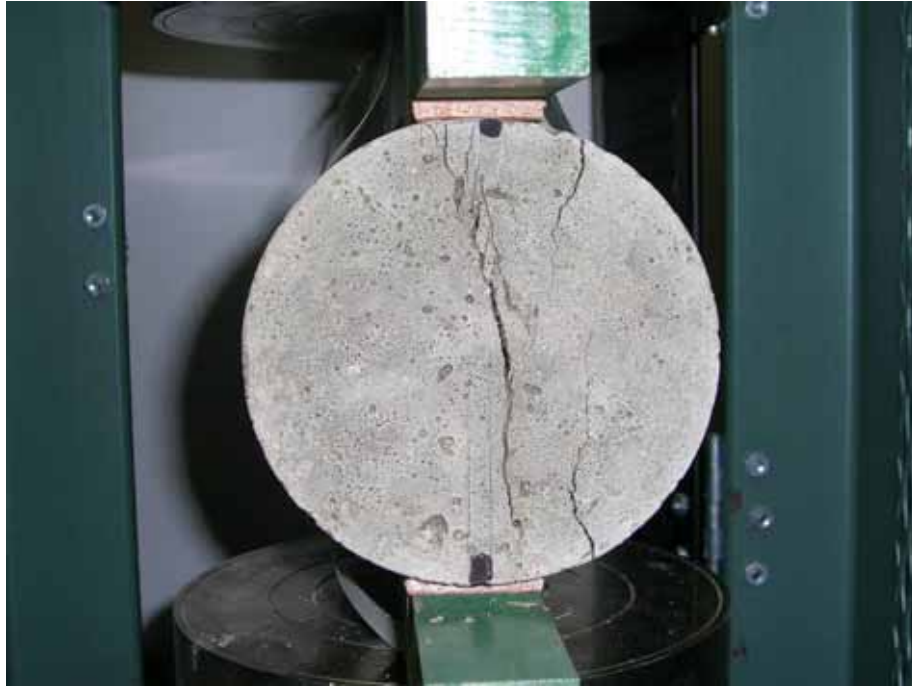
Figure 8. PCC splitting tensile strength test
