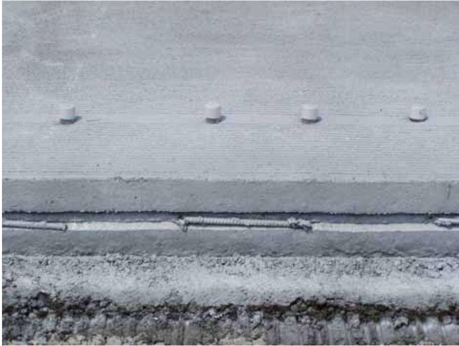
Figure G.11. Hygrochron relative humidity instrumentation
