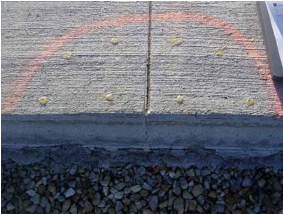
Figure D.14. Corner DEMEC location with crack at transverse joint
