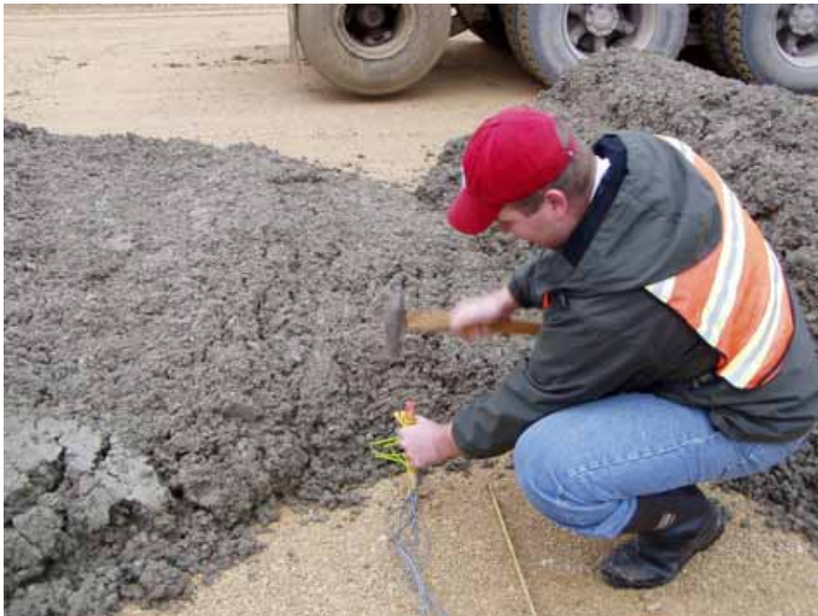
Figure A.14. Temperature instrumentation installation
