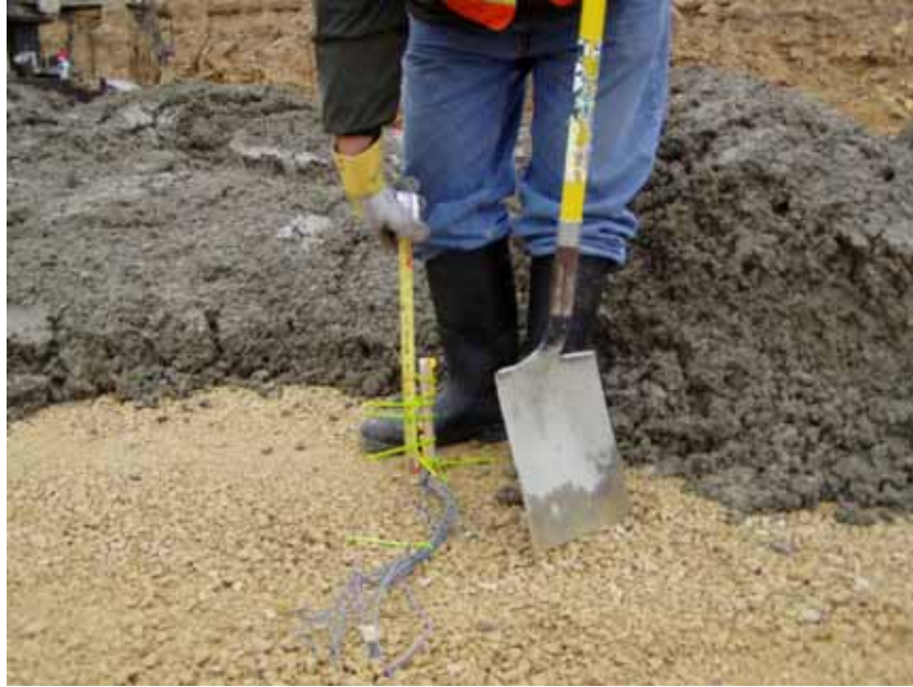
Figure 18. Typical temperature instrumentation
