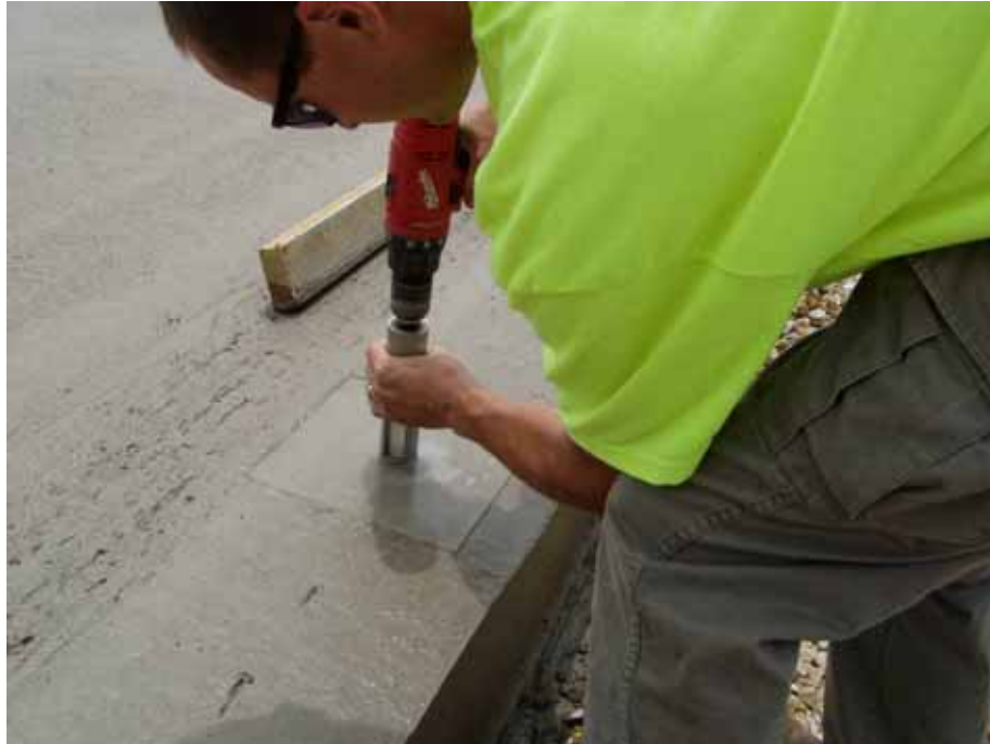
Figure D.9. Air Void Analyzer (AVA) sampling
