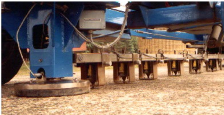
**Figure 2. FWD bottom view with sensor locations (Source: [http://training.ce.washington.edu/WSDOT/Modules/09\\_pavement\\_evaluation/09-5\\_body.htm](http://training.ce.washington.edu/WSDOT/Modules/09_pavement_evaluation/09-5_body.htm))**
