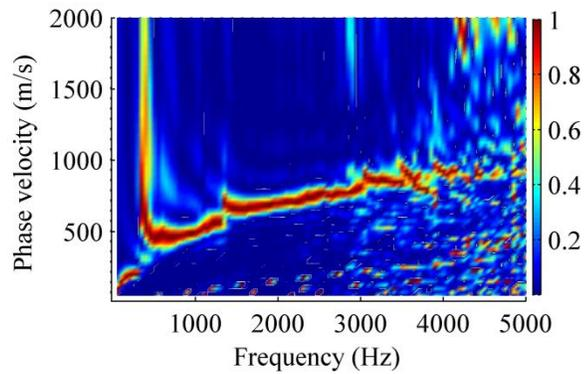
**Figure A.3. Results of surface wave tests on ambient-temperature Boone HMA base courses one day after paving. Left column: normalized time-domain signals, right column: frequency-domain dispersion images**
