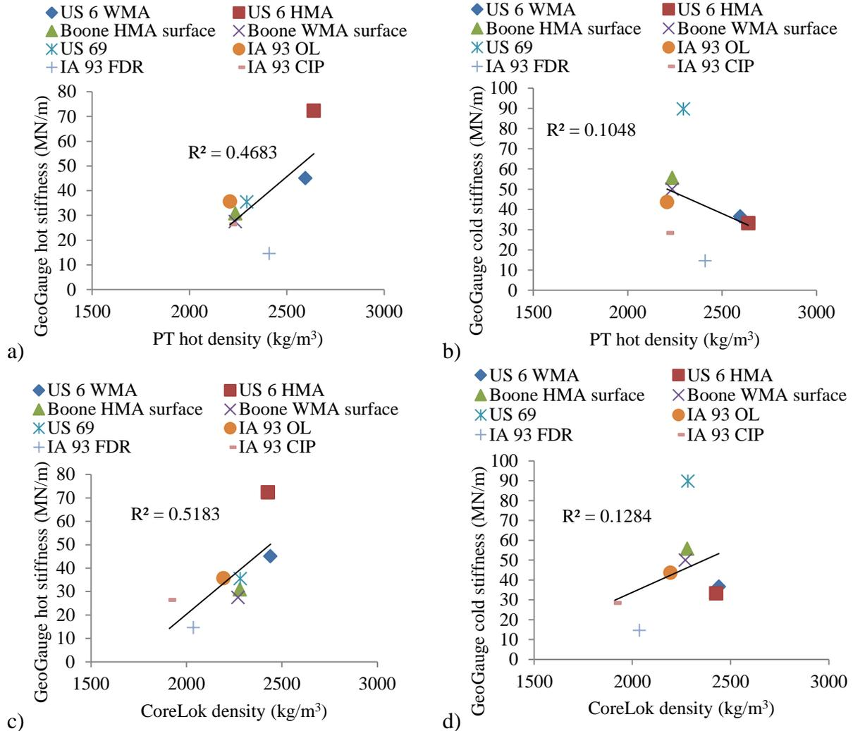
**Figure 5.5 Correlation between GeoGauge stiffness and density: (a) hot GeoGauge and hot PT tests, (b) cold/ambient GeoGauge and hot PT tests, (c) hot GeoGauge and CoreLok tests, (d) cold/ambient GeoGauge and CoreLok tests**
