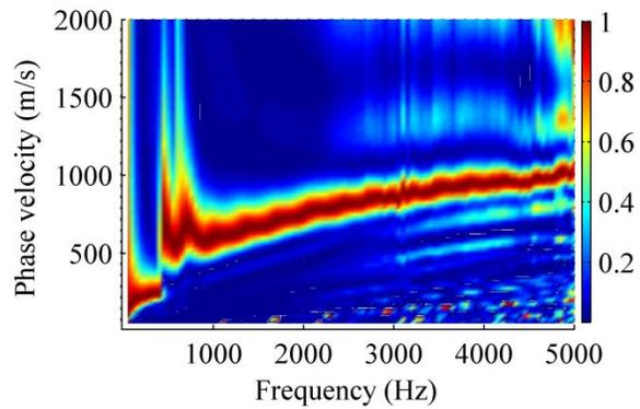
**Figure A.4. Results of surface wave tests on ambient-temperature Boone WMA base courses one day after paving. Left column: normalized time-domain signals, right column: frequency-domain dispersion images**
