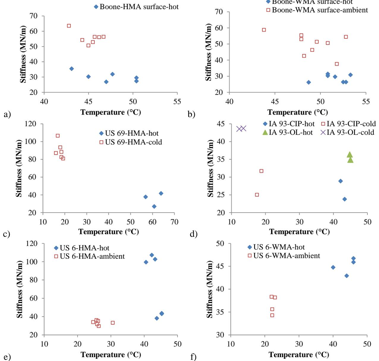
**Figure 3.14. GeoGauge stiffness measurements: (a) Boone HMA surface course, (b) Boone WMA surface course, (c) US 69 HMA section, (d) IA 93 CIP and OL sections, (e) US 6 HMA section, and (f) US 6 WMA section**
