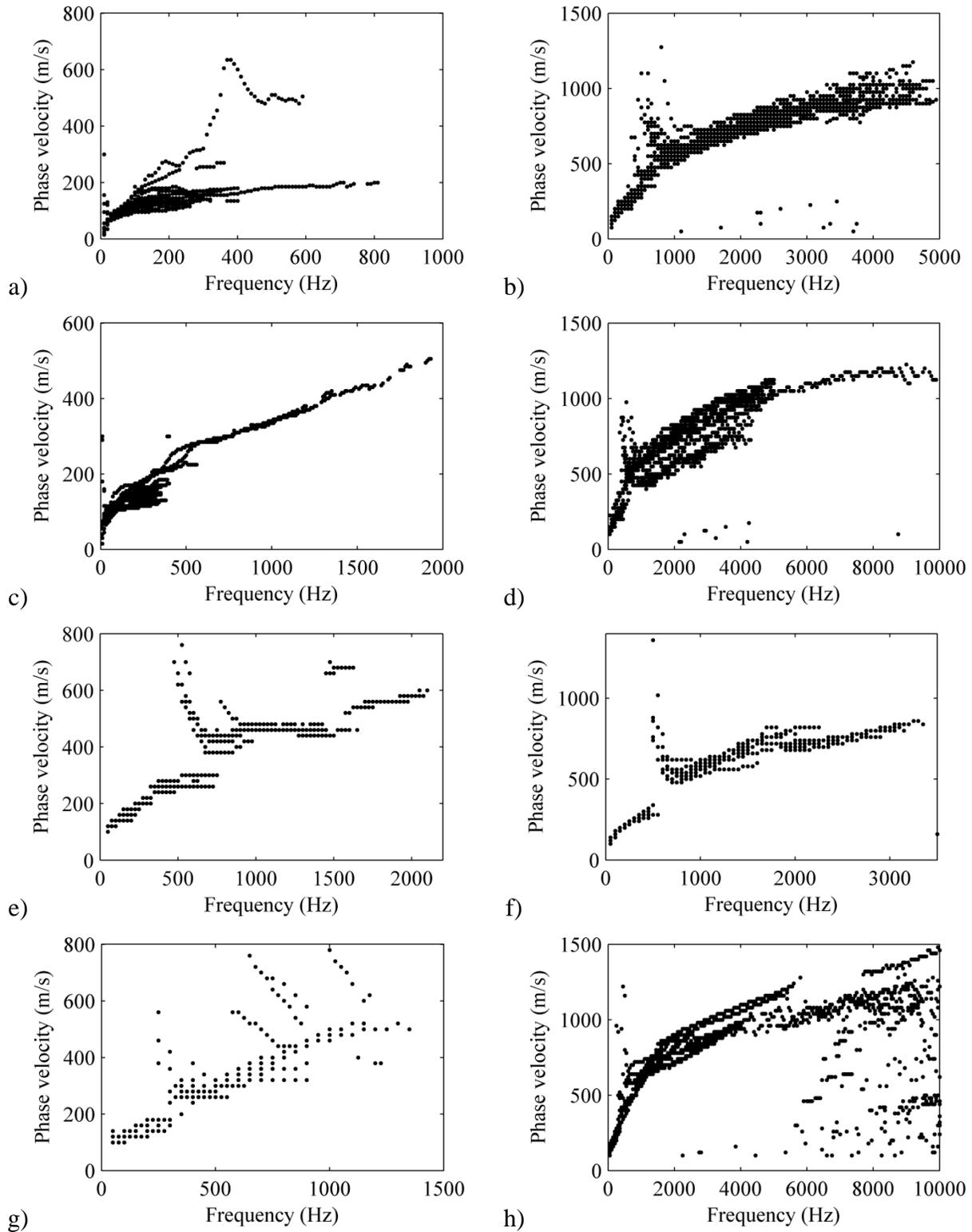
**Figure 3.4. Dispersion trends of Boone HMA base courses: (a) several hours after paving, (b) several days after paving; Boone WMA bases: (c) several hours after paving, (d) one day after paving, Boone HMA surface: (e) several hours after paving, (f) one day after paving; Boone WMA surface: (g) several hours after paving, (h) several days after paving**
