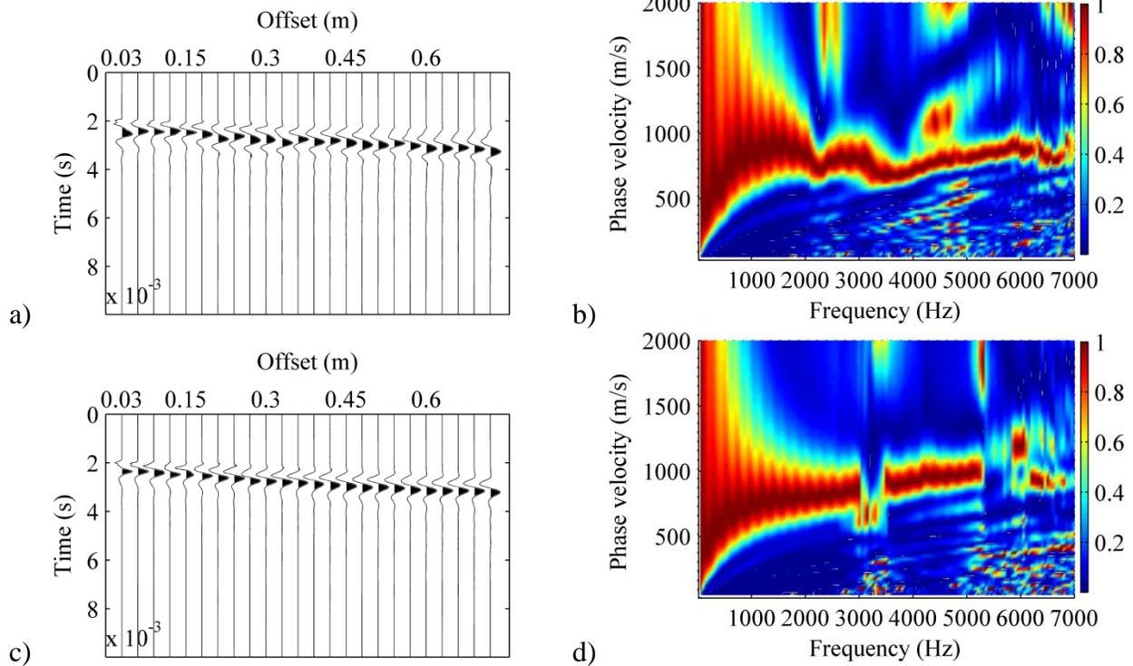
**Figure 3.5. MSOR surface-wave test results at location US 69-9: (a) normalized time-domain data for hot test, (b) experimental dispersion trend for hot test, (c) normalized time-domain data for cold test, (d) experimental dispersion trend for cold test**
