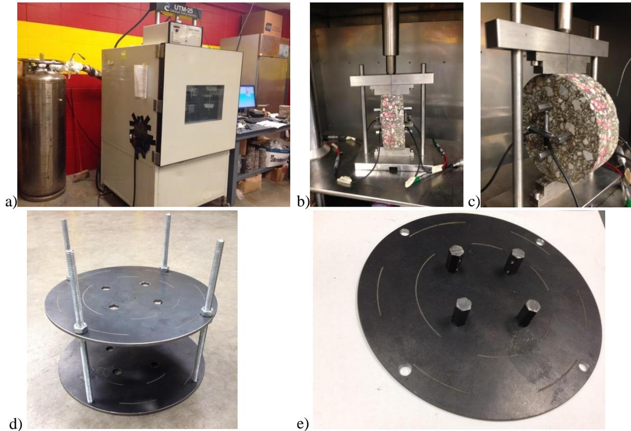
**Figure 2.11. Indirect tension test setup: (a) full view, (b) 4 in. core with two LVDTs on each side in the chamber, (c) horizontal and vertical LVDTs mounted on one side of a 4 in. core, (d) custom-built alignment jig for installation of LVDT targets, (e) bottom plate of jig with four LVDT targets.**
