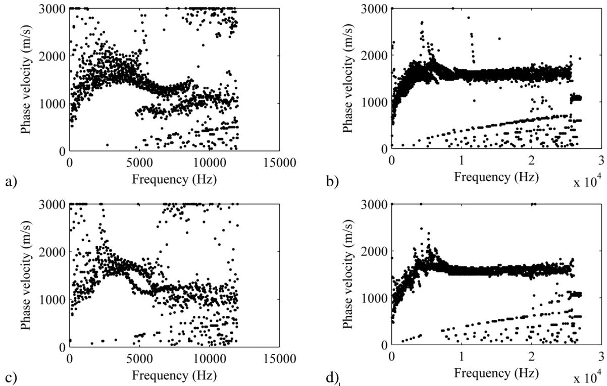
**Figure 3.12. Dispersion trends of US 6 HMA surface course: (a) several hours after paving, (b) several days after paving; and US 6 WMA surface course: (c) several hours after paving, (d) several days after paving**
