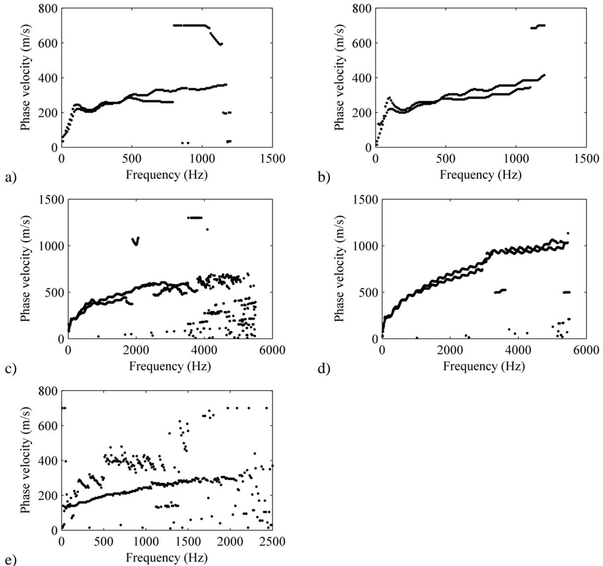
**Figure 3.10. Dispersion trends of IA 93 sections: CIP section (a) several hours after paving, (b) several hours after paving and using dry ice; OL section: (c) several hours after paving, (d) several hours after paving and using dry ice; FDR section: (e) several hours after paving**
