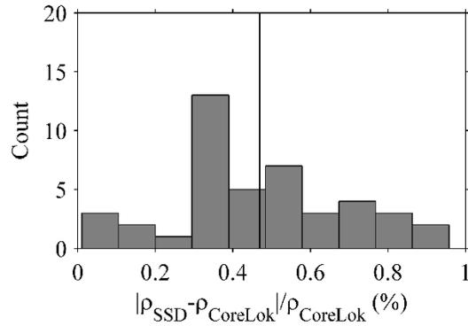
**Figure 4.3. Density difference between CoreLok and SSD densities**
