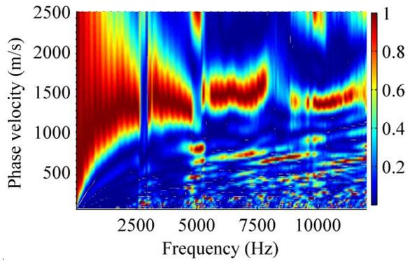
**Figure A.15. Results of surface wave tests on ambient-temperature US 169 HMA surface course two days after paving. Left column: normalized time-domain signals, right column: frequency-domain dispersion images**
