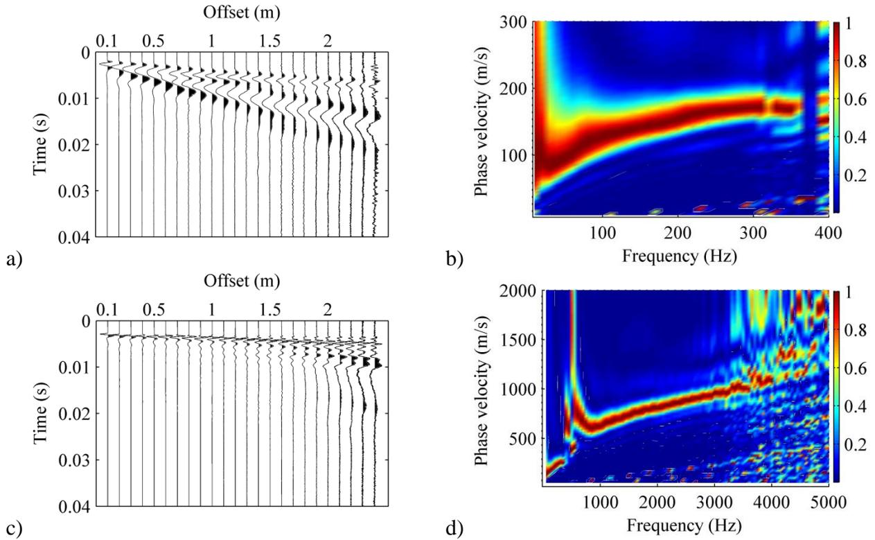
**Figure 3.3. MSOR surface-wave test results for Boone HMA base course location HB1-1: (a) normalized time-domain data for hot test, (b) experimental dispersion image for hot test, (c) normalized time-domain data for ambient-temperature test, (d) experimental dispersion image for ambient-temperature test**
