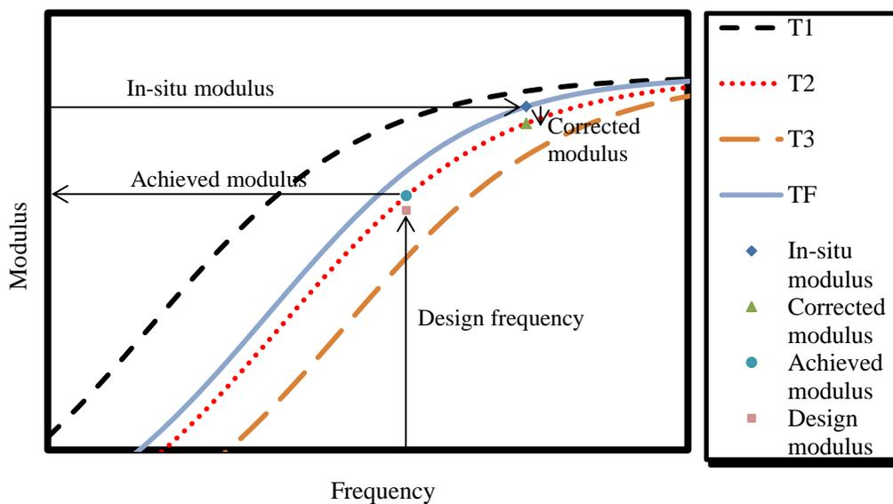
**Figure 5.7 Quality assurance procedure based on NDT measurements**
