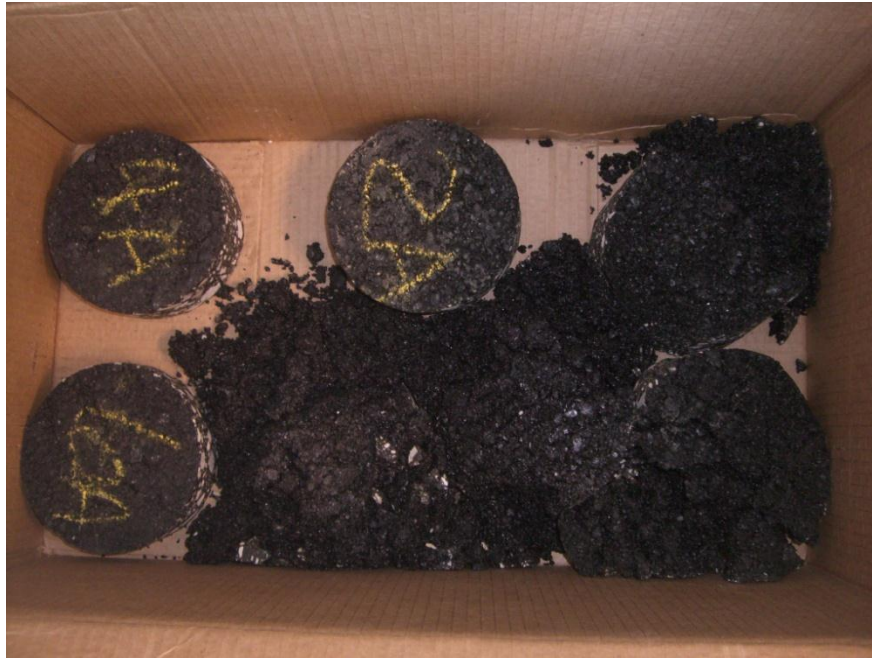
Figure 5.2. Deterioration of Safety Edge core samples from Jasper County
