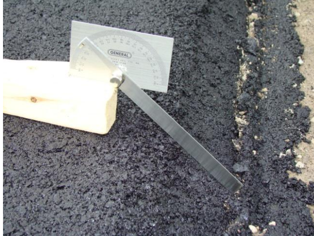
Figure 4.1. Slope-measuring tool developed by CTRE
