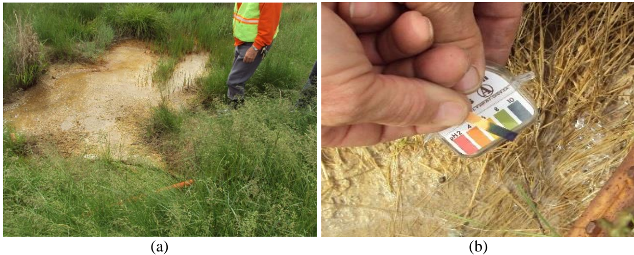
Figure 11. Vegetation condition in the vicinity of drain outlets carrying tufa materials (I-35/N/MP141.30): (a) vegetation kill (dead zone), (b) water from the drainage outlet pipe showing a pH value of 10
