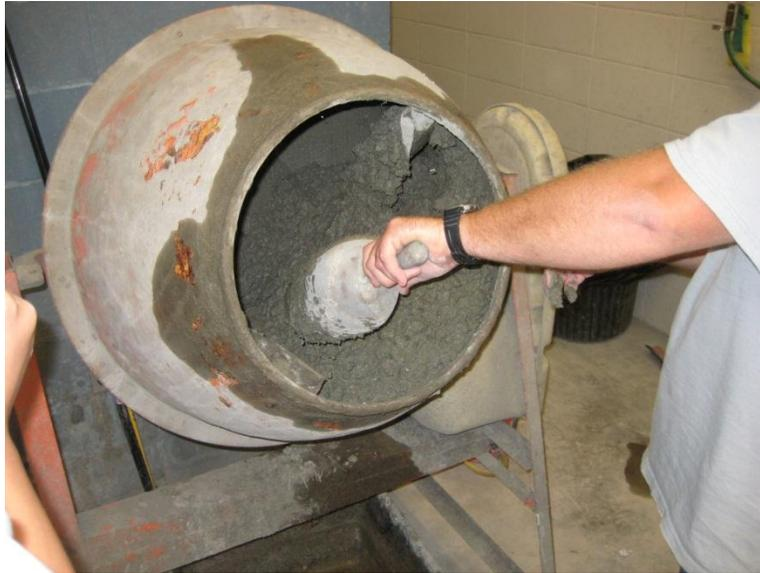
**Figure 28. Preparation of concrete mix**
