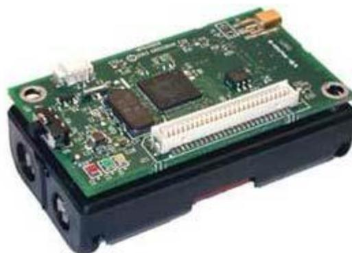
**Figure 15. Mote (MEMS) sensor (Kim et al. 2006)**
