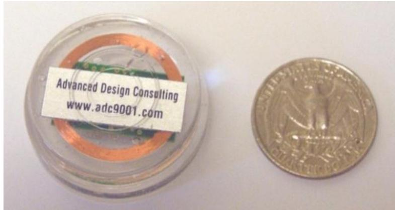
**Figure 3. ADC's MEMS concrete monitoring system (ADC)**
