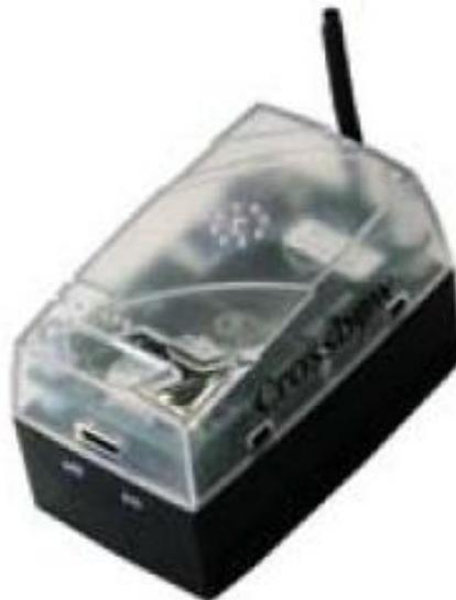
**Figure 9. Crossbow sensor node with sensor board (Crossbow Technology, Inc. 2007)**
