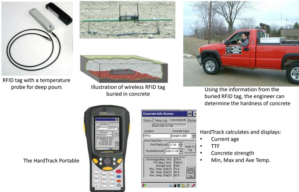
**Figure 52. RFID-based wireless concrete monitoring system (WAKE, Inc.)**
