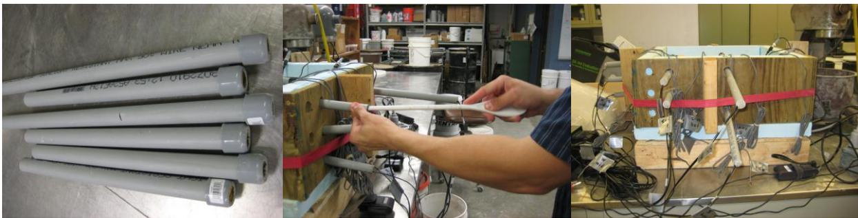
**Figure 26. MEMS sensor installation in concrete slab form**
