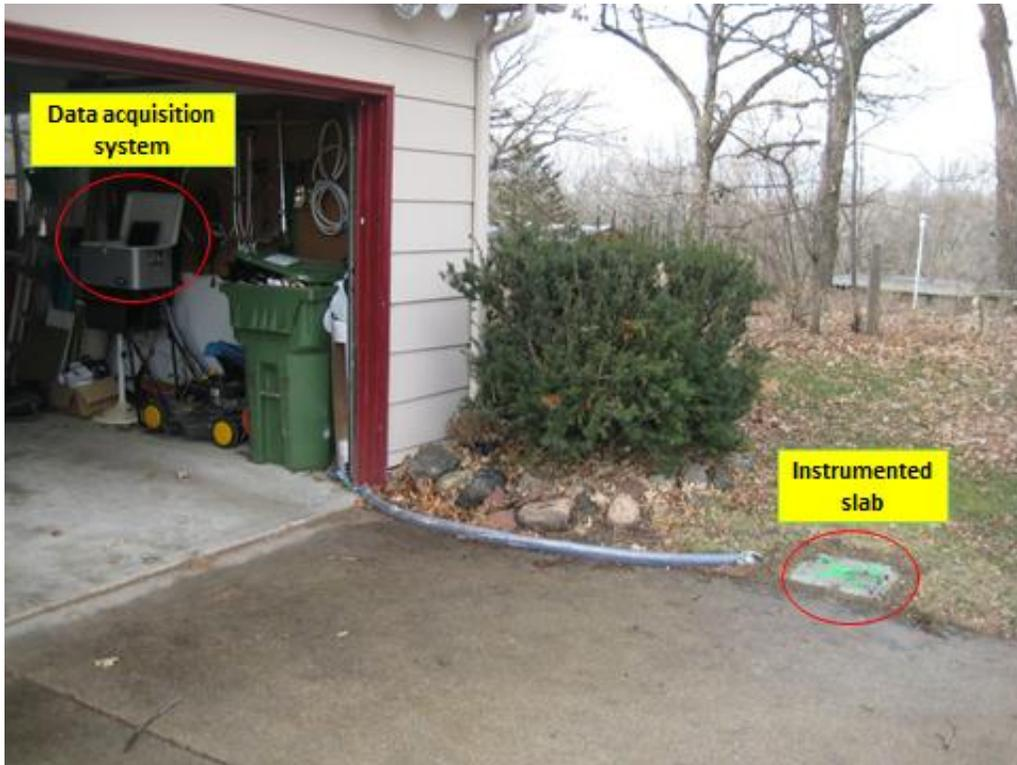
**Figure 46. Instrumented slab near driveway in Ames, Iowa during test phase 4**
