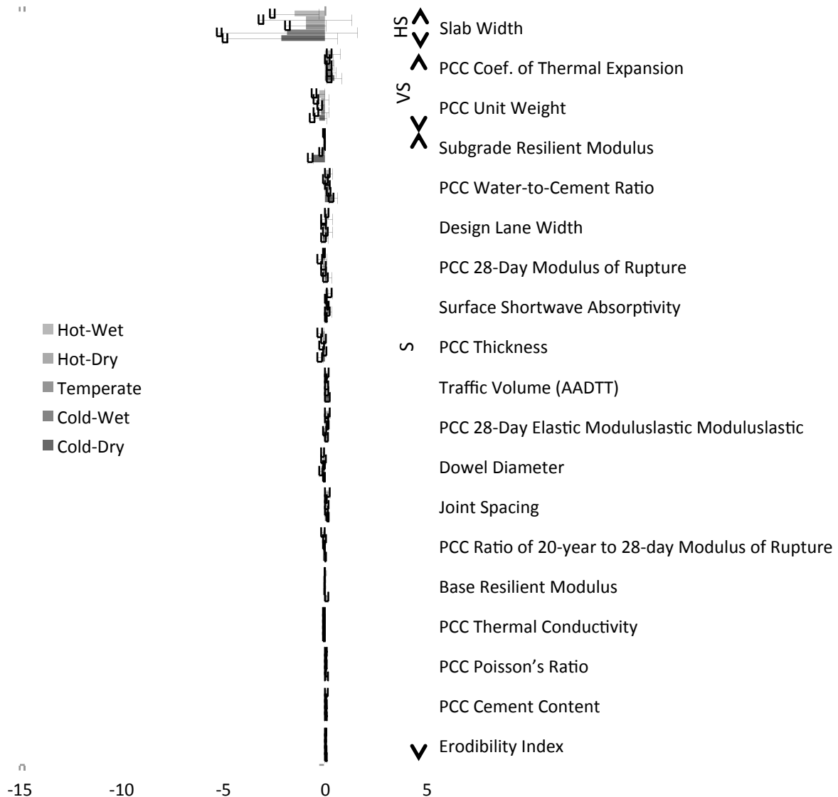
Figure 10.14. Ranking of New JPCP design inputs by |\mu \pm 2\sigma| NSI values: IRI.
