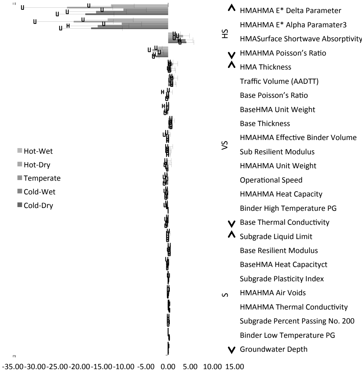
Figure 9.18. Ranking of HMA Over Stiff Foundation design inputs by |\mu \pm 2\sigma| NSI values: AC rutting.
