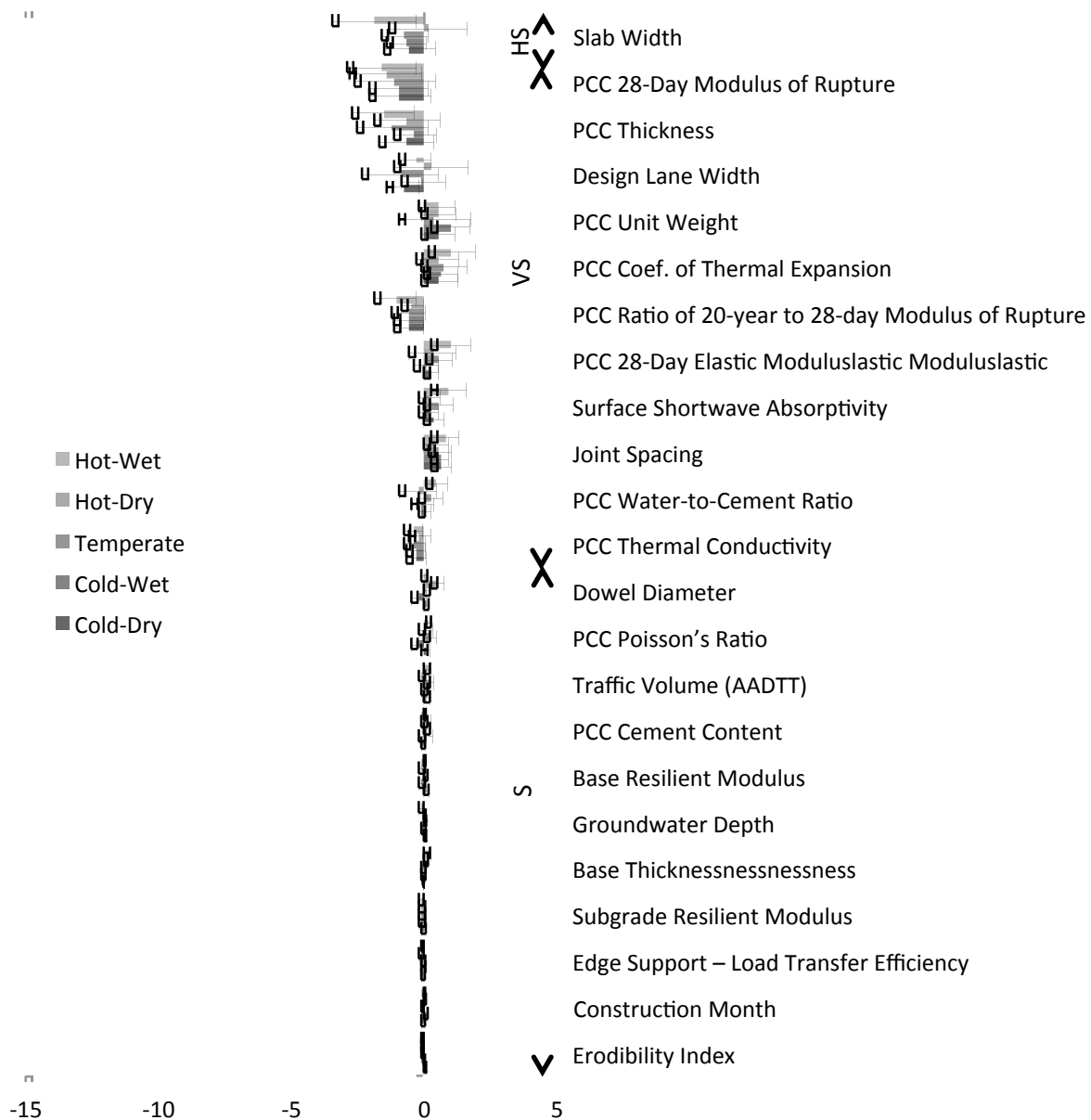
Figure 10.13. Ranking of New JPCP design inputs by |\mu \pm 2\sigma| NSI values: transverse cracking.
