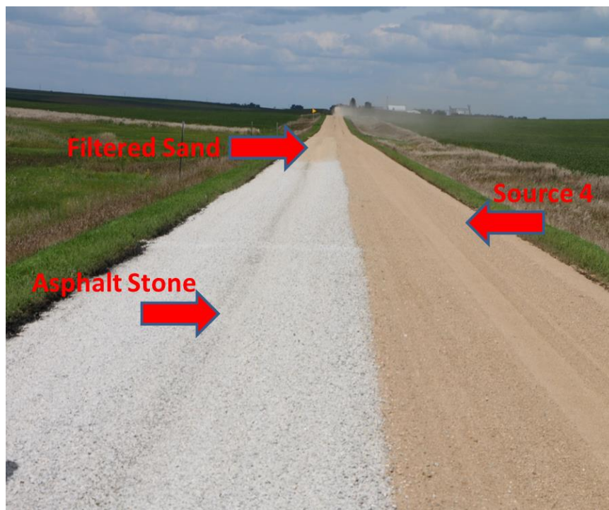
Figure 52. Source 4 aggregate (TS 4), asphalt aggregate (TS 1), and filter sand (TS 2)
