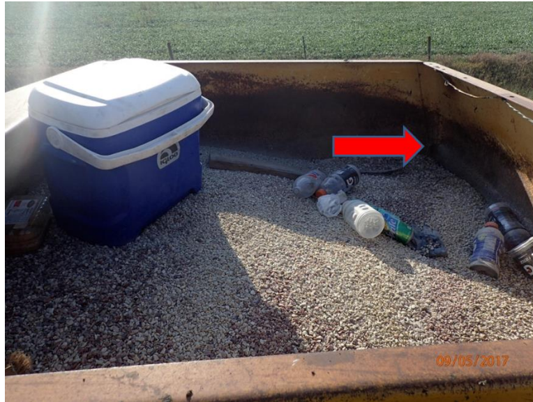
Figure 54. Roller was not filled to the required weight for first layer construction
