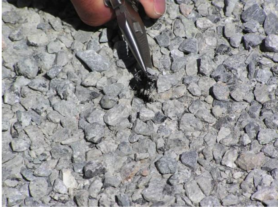
Figure 6. The goal is to achieve 70 percent chip embedment into the binder
