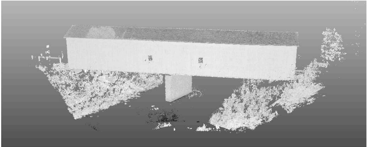
Figure 3A.--A point cloud image from the Zumbrota bridge created from a single exterior scan processed with Faro Scene software
