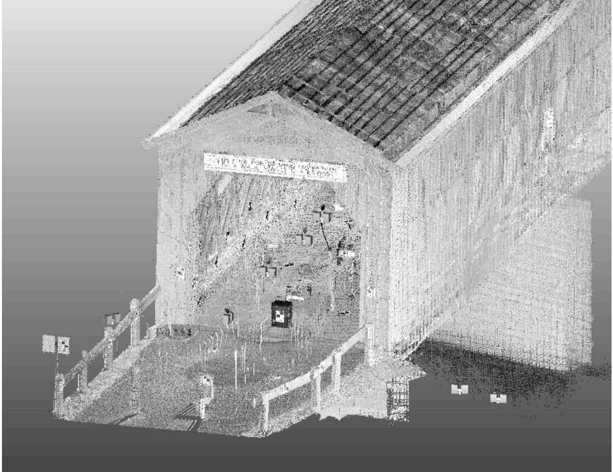
Figure 5.--A point cloud image of the Zumbrota bridge created from multiple scans and linked together with Faro Scene software.
