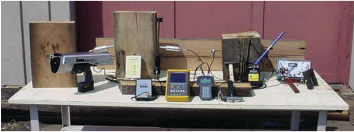
Figure 10.4—Various tools and techniques available to conduct condition assessments (used with permission of Natural Resources Research Institute, University of Minnesota Duluth, Brashaw et al. 2005b).
