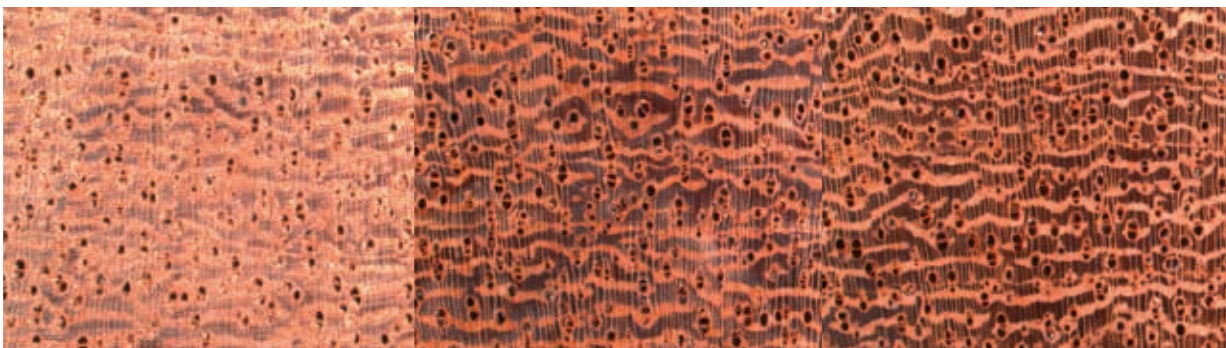
Figure 4.8—Cuts of different quality. The left image shows the specimen cut with a sharp table saw. The middle image shows the specimen cut cleanly with a utility knife. The right image shows the specimen prepared in a laboratory, resulting in a research-quality image.
