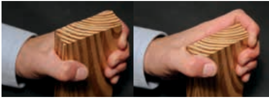
Figure 4.5—The correct grip for holding a specimen for cutting (left). Note that the fingers and thumb are below the top of the specimen and will not be cut. On the right, the specimen is held with the fingers and thumbs in a way that will result in injury when the specimen is cut.
