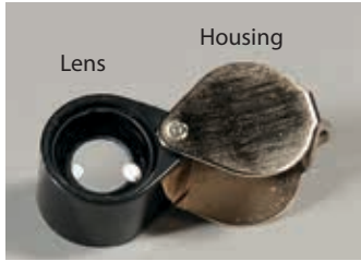
Fig. 3.1—A hand lens has two main parts, the lens and the housing.
