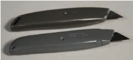
Figure 4.3—The preferred basic tool for cutting wood, utility knives will make clean cuts of all but the softest woods.
