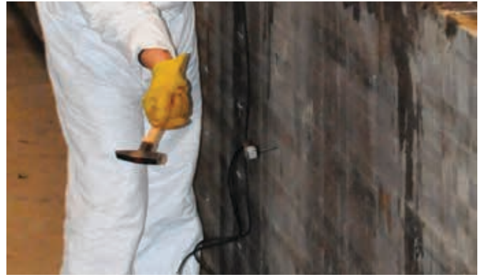
Figure 10.8—Transverse stress wave velocity measurement method.
