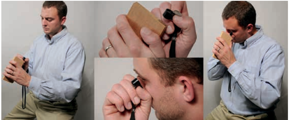
Figure 3.2—Using a hand lens to observe a wood specimen. On the left, the distance between the lens and the observer’s eye is much too great, but the distance between the lens and wood specimen is correct. The top photo in the center shows the correct distance between the lens and the wood specimen. The bottom photo in the center shows the correct distance between the lens and the eye. The photograph on the right shows the correct distances between the lens, the specimen, and the eye.
