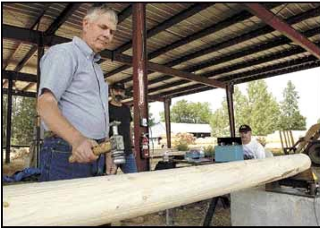
Figure 17—Determination of modulus of elasticity by transverse vibration of lodgepole pine logs at Portbuilt, Inc., Hamilton, Montana, in July 2004.
