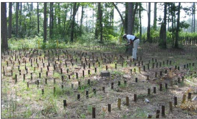
Figure 2—Wood preservative formulations undergo rigorous testing, including lengthy field trials.
