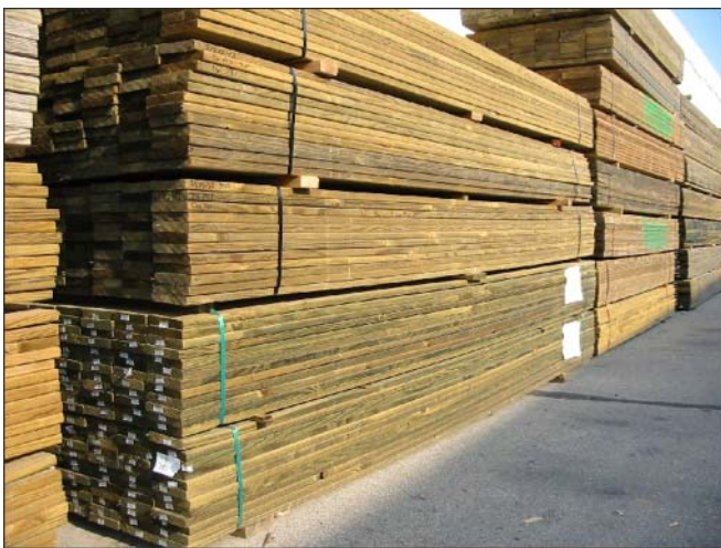
Figure 8—Stacks of ACQ-C and CA-B treated lumber await sale at a lumberyard. Multiple retentions are available for different end-uses.
