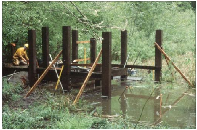
Figure 6—Evaluation of ACQ-B treated wetland boardwalk for leaching and environmental impact.
