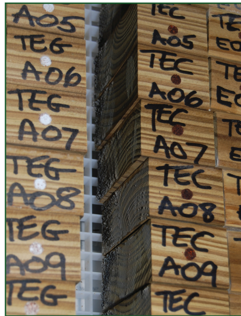
Hot-dip galvanized (left) and common steel (right) fasteners exposed to treated wood during a 1-year exposure at 27°C, 100% relative humidity.
