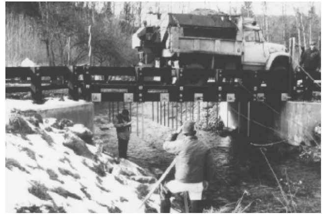
Figure 15—Load test 1 bridge deflections were measured by suspending calibrated rules from the deck underside and reading displacement values with a surveyor's level.
