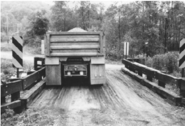
Figure 17—Load test 2 transverse load positions (looking north): (top) load position 1; (middle) load position 2; (bottom) load position 3. For all load positions, the two rear axles were centered over the bridge midspan with the front axle off the span.
