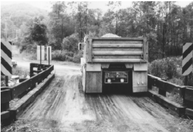
Figure 18—Load test 2 was measured with string potentiometers and an electronic data acquisition system.
