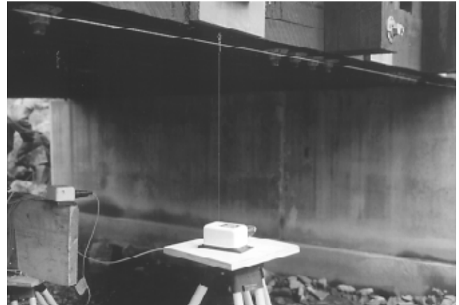
Figure 18—Load test 2 was measured with string potentiometers and an electronic data acquisition system.
