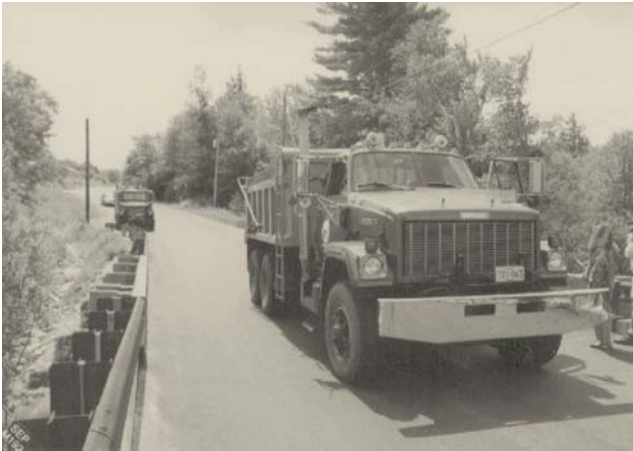
Figure 18—One of the two trucks used for load test 1.
