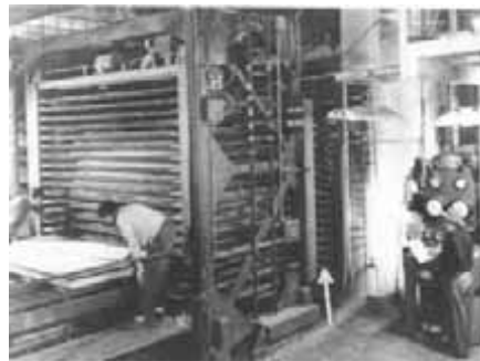
Figure 43.— Glued and assembled veneers being transferred to automatic press loader. Arrow points to 20-opening steam-heated hot press.
