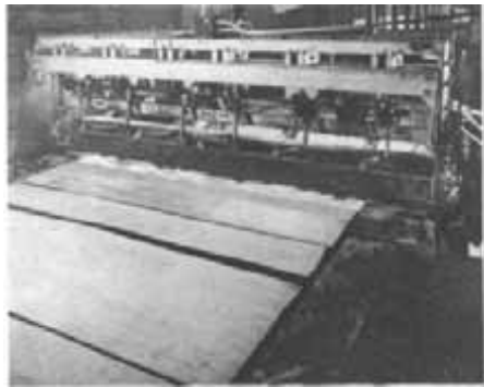
Figure 39.— Clipping softwood veneer to width and cutting out objectionable defects.
