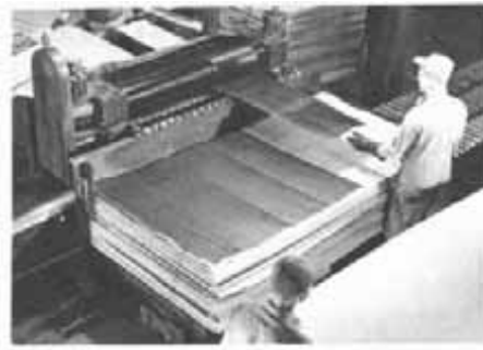
Figure 41.— Spreading glue on veneer with a conventional double-roll glue spreader and assembling the veneers for plywood.
