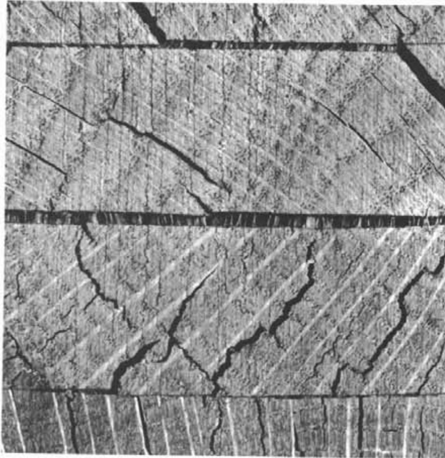
Figure 14.— Cross section of laminated oak glued with thermosetting or cross-linked PVA and subjected to vacuum-pressure soaking, steaming, and drying. The bridging in the joint at the center might explain why PVA glues have performed well in cyclic tests on mortise and tenon and dowel joints. Had a brittle glue been used, fractures would probably have occurred either in the bond or adjacent to the glueline. The elastic PVA yielded enough to retain the bond between the joint surfaces.
