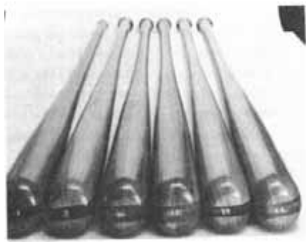
Figure 73.— Laminated baseball bats with center lamination of hickory for improved impact strength and the remaining sections of ash with edge grain exposed on the surface of the bat. Edge-grained surfaces make the bat more resistant to shelling.
