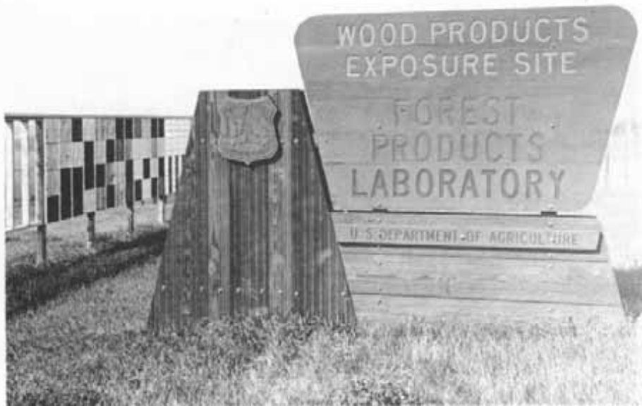
Figure 11.— Test fence for evaluation of glue-bond durability in plywood. The Forest Service maintains four such test areas to determine durability of adhesives under different climatic conditions. One test area is near Madison, Wis.; one south of Olympia, Wash.; one at San Joaquin Experimental Range, Calif.; and the fourth at the Harrison National Forest, La. Various types of glued wood products are exposed at each site.
