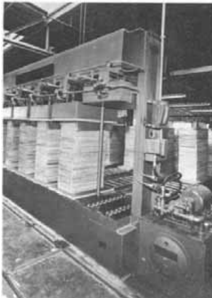
Figure 64.— Cold-pressing panels for cabinet doors glued with modified PVA.
