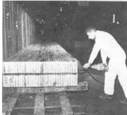
Figure 52.— Tightening clamps on glued assemblies with nut runner operated by compressed air.
