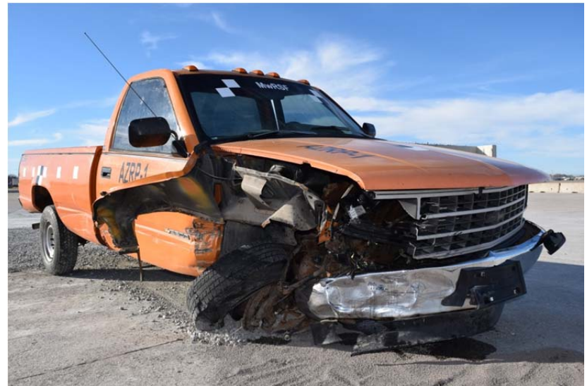
FIGURE 5 Vehicle damage and barrier damage, Test AZRP-1.
