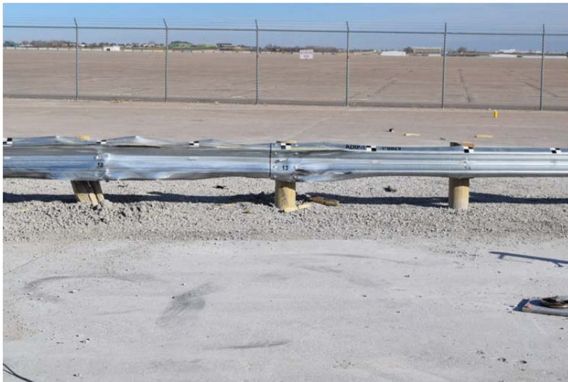
FIGURE 5 Vehicle damage and barrier damage, Test AZRP-1.
