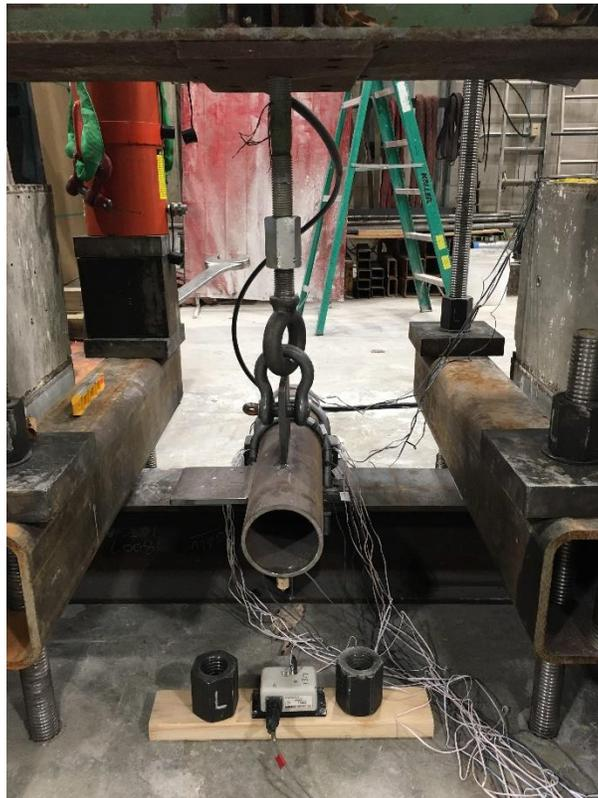
(b) Type-A specimen subjected to vertical load
