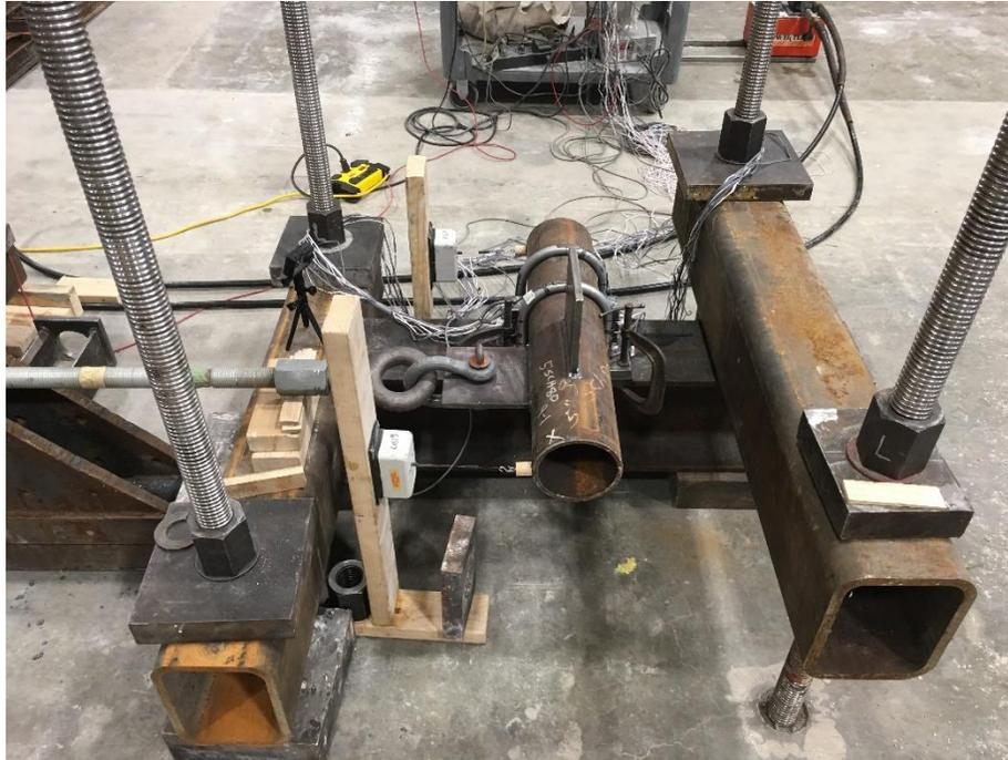
(a) Type-A specimen subjected to horizontal load
