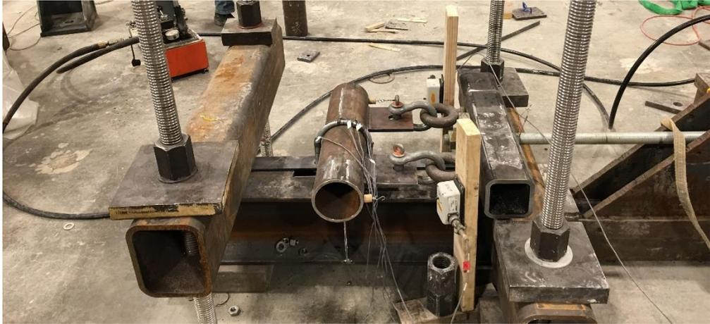
Figure 25. Type-B specimen setup before testing
