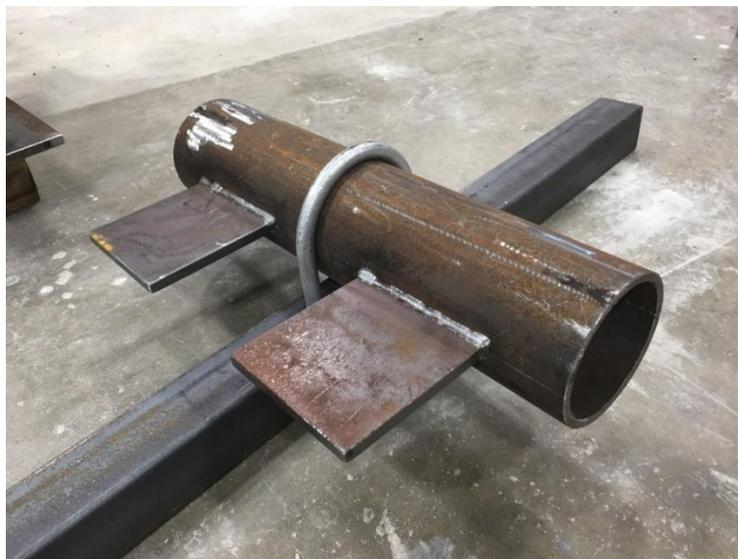
**Figure 23. Type-B specimen**
