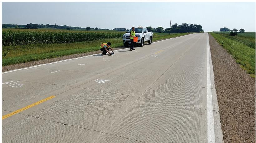
*Joint activation data being collected on an existing overlay in Worth County, Iowa using a MIRA device placed over the sawcuts*
