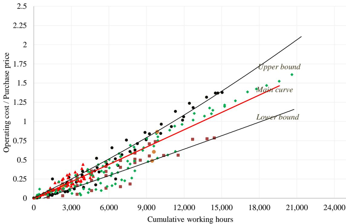
**Figure 5.12. Grader regression model and the upper and lower bond on the grader data set**
