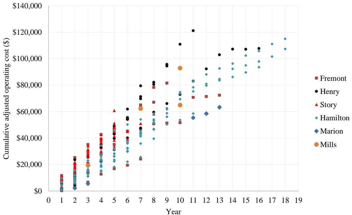
**Figure 5.8. Age-based adjusted operating cost of the motor grader database**
