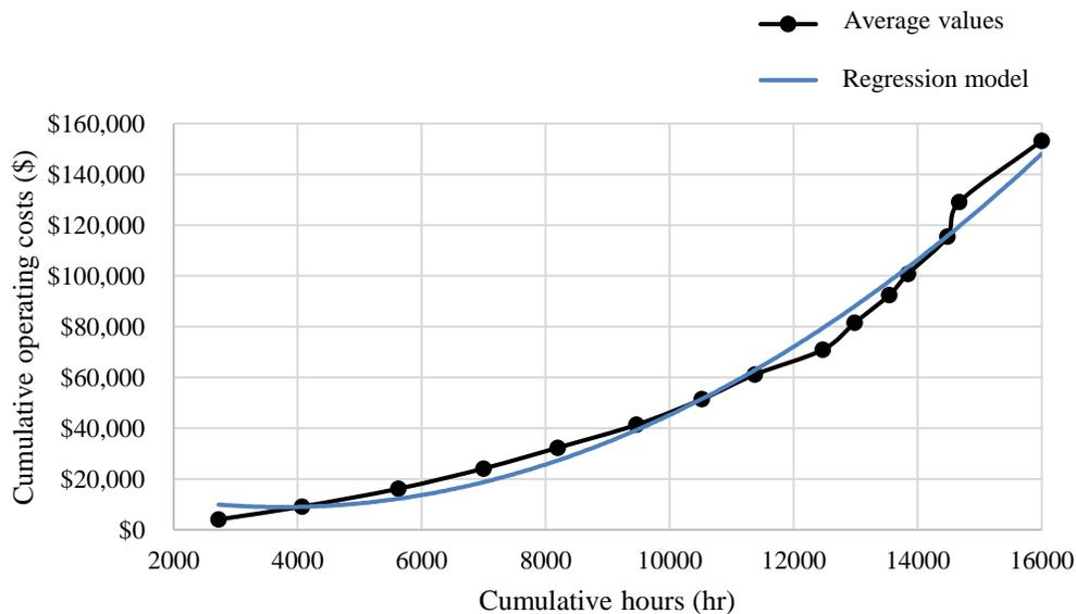
**Figure 2.3. Relationship between hours and operating costs for tandem-axle trucks**
