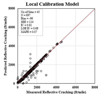
Measured versus predicted reflective cracking for a nationally calibrated model (top) and a locally calibrated model (bottom)
