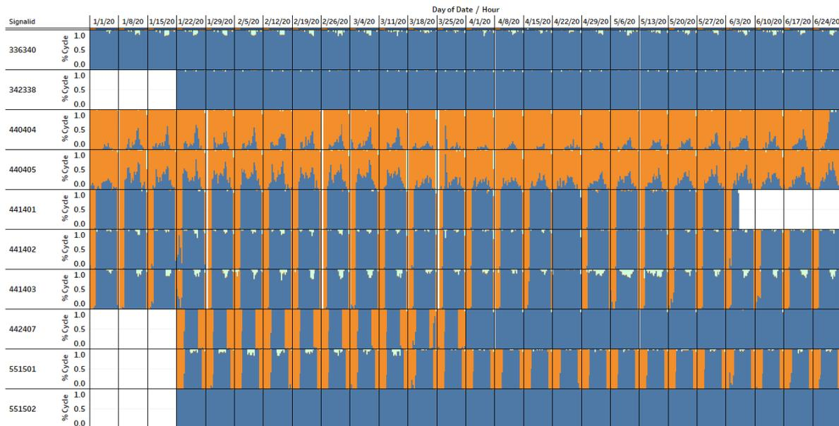
**Figure 26. Examples of phase 2 termination for identifying coordinated phases**
