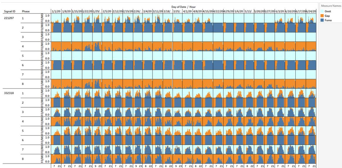
**Figure 25. Distribution of phase terminations by date, and by phase, at two intersections**
