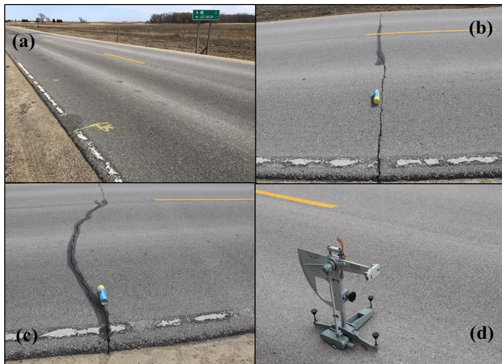
Figure 20. Field survey on March 22, 2018: (a) control section, (b) treated section No. 1 (0.03 gal/yd 2 ), (c) treated section No. 2 (0.025 gal/yd 2 ), and (d) treated section No.3 (0.02 gal/yd 2 )
