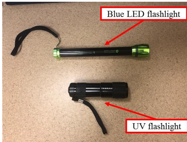
Figure 8. Flashlight for measurements of penetration depth
