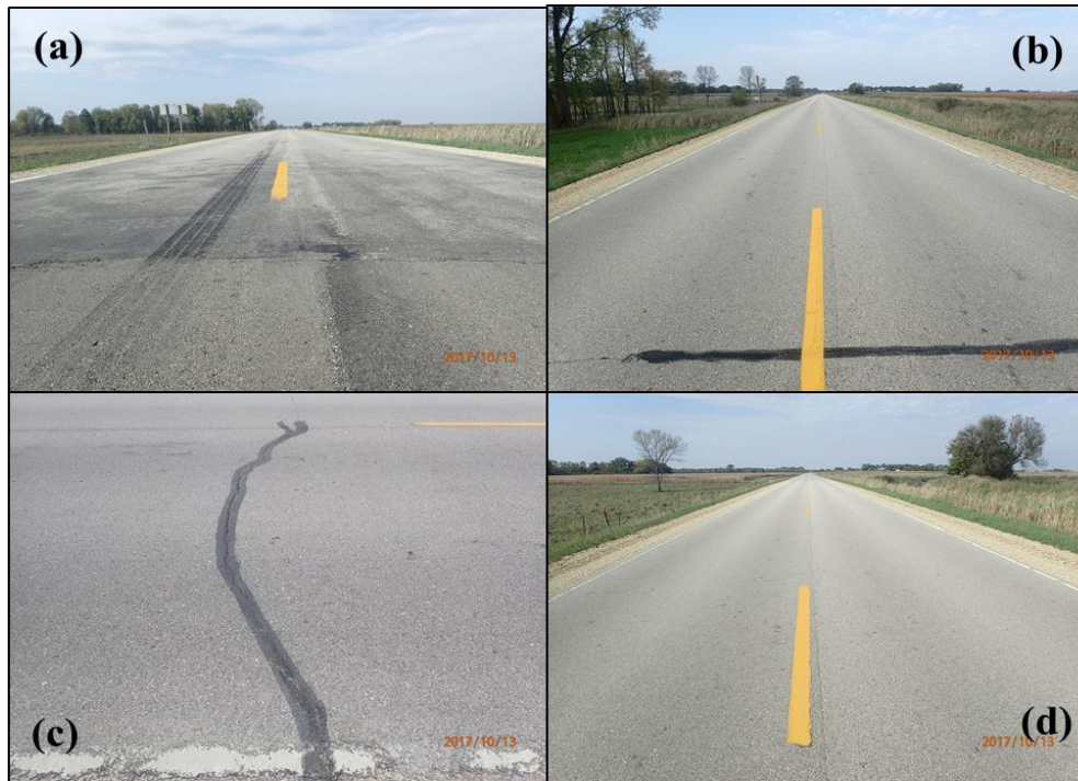
Figure 19. Field survey on October 13, 2017: (a) control section, (b) treated section No. 1 (0.03 gal/yd 2 ), (c) treated section No. 2 (0.025 gal/yd 2 ), and (d) treated section No.3 (0.02 gal/yd 2 )
