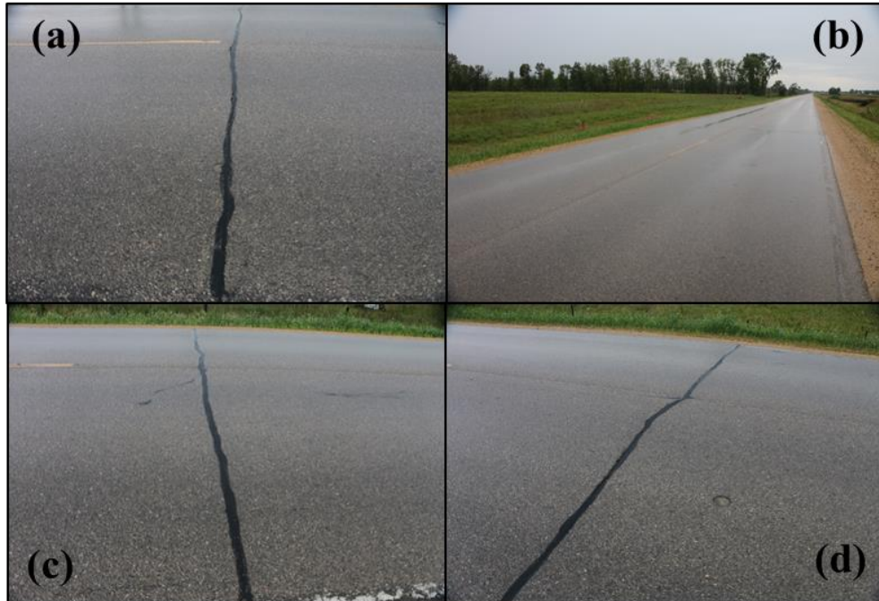
Figure 23. Field survey on August 24, 2021: (a) control section, (b) treated section No. 1 (0.03 gal/yd 2 ), (c) treated section No. 2 (0.025 gal/yd 2 ), and (d) treated section No.3 (0.02 gal/yd 2 )
