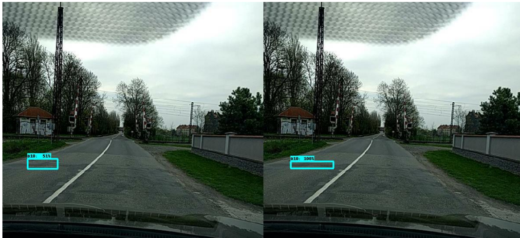
Figure 35. Transverse crack distress detection by SSD 320
