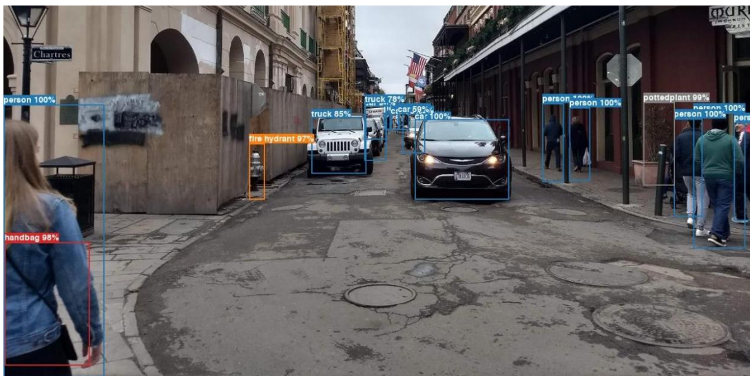
Figure 26. Example of object detection using a deep-learning model
