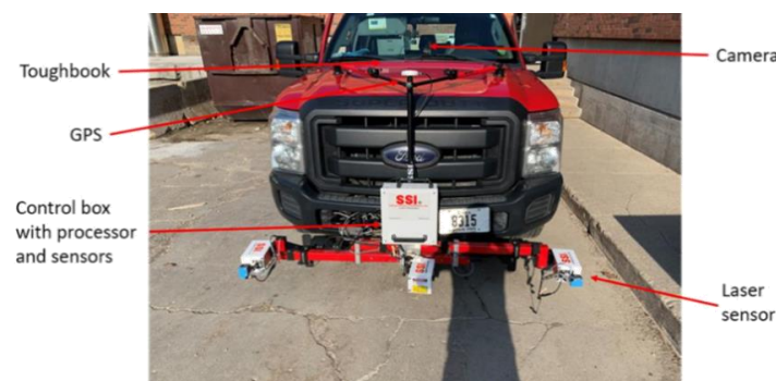
Figure 2. Class 1 high-speed profilometer for IRI measurement
