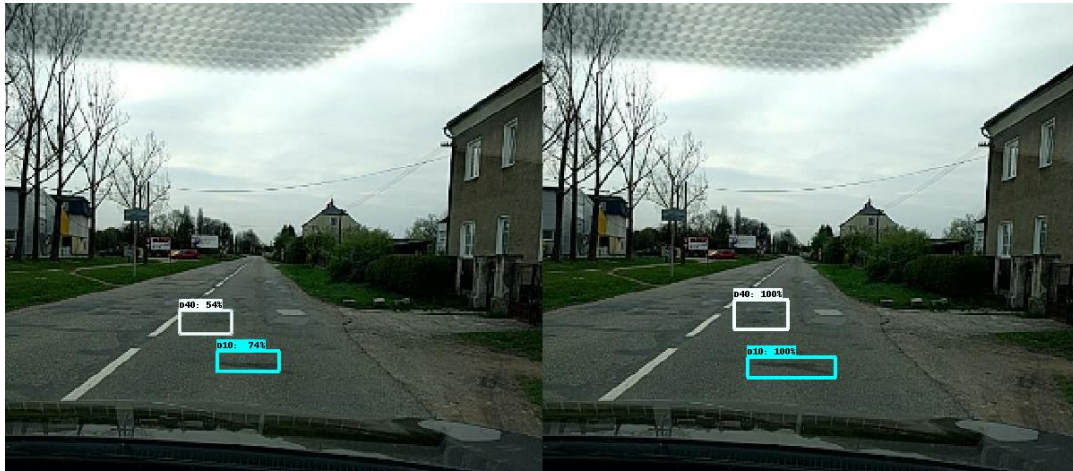
Figure 32. Pothole and transverse crack distress detection by SSD 640
