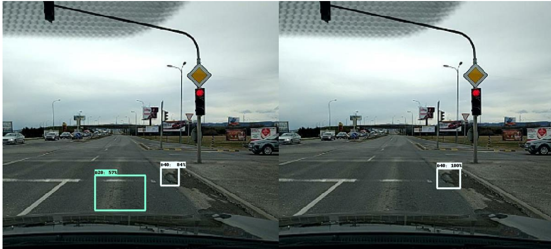
Figure 34. Pothole and alligator crack distress detection by SSD 640
