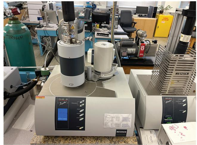
Thermogravimetric test equipment
