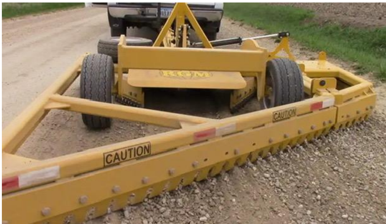
Figure 85. Gravel rake used to retrieve coarse aggregates from shoulders
