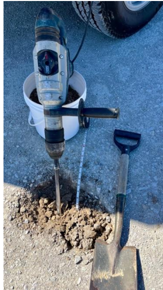
Figure 84. Method of collecting surface samples using hammer drill with chisel bit
