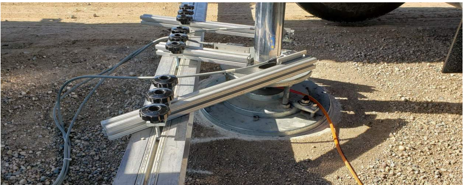
Figure 3. Picture of APLT setup with 18 in. diameter loading plate (Picture taken on 05/27/2022 at 05:18pm)
