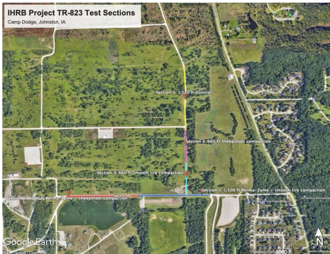
Figure 31. Project test section layout
