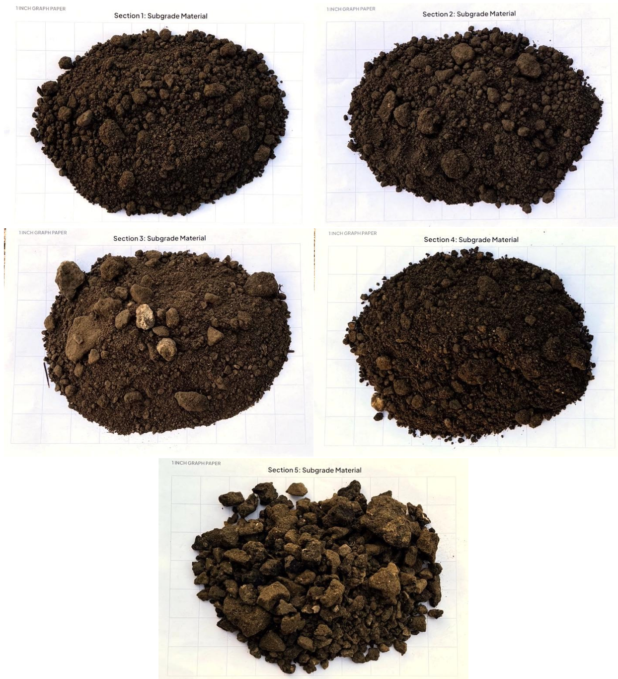
Figure 12. Subgrade samples collected from each test section during construction
