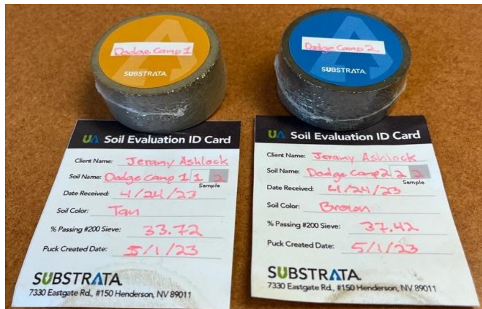
Figure 32. Soil samples from project site treated with Perma-Zyme stabilizer
